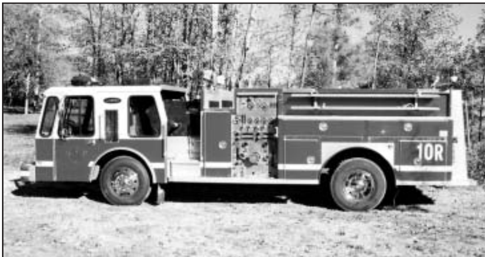
1985 E-ONE HURRICANE 1250 HALE PUMP 500 GALLON TANK
