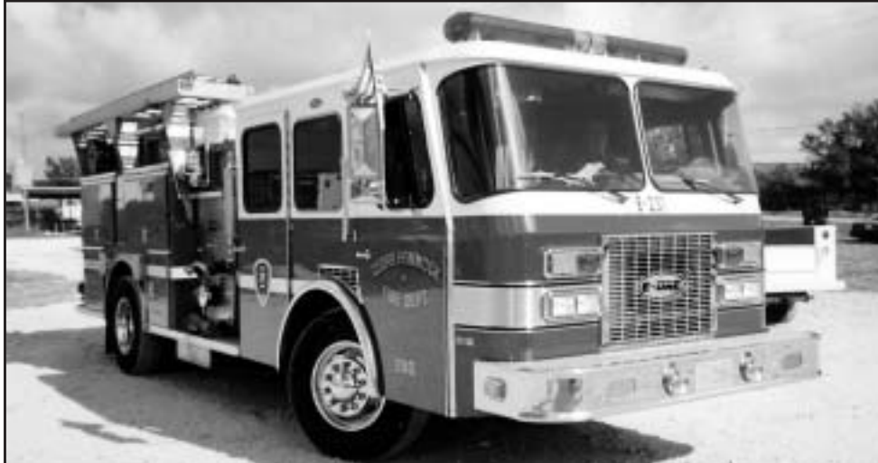
1992 E-ONE PROTECTOR 1250 TOP MOUNT HALE PUMP 1000 GALLON TANK
