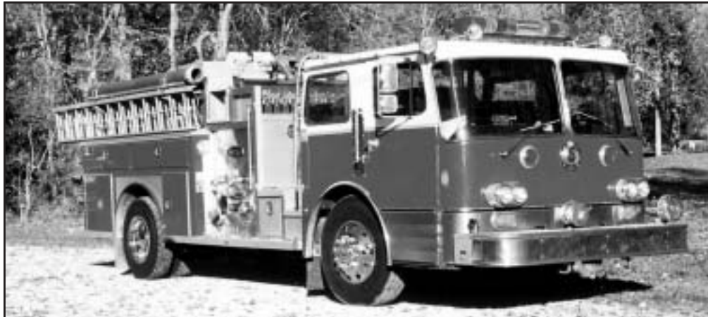
1983 E-ONE PEMFAB 1250 HALE (TOP-MOUNT) PUMP 750 GALLON TANK
