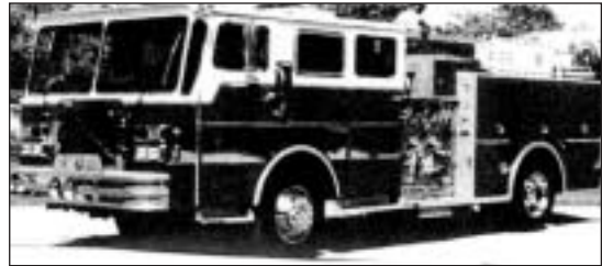
1984 Spartan Pumper 8 Man Cab Diesel / Automatic 1500 Pump / 1000 Tank
