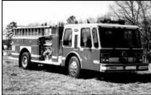
1985 E-ONE HURRICANE 1250 HALE PUMP 500 GALLON TANK DIESEL AUTOMATIC
