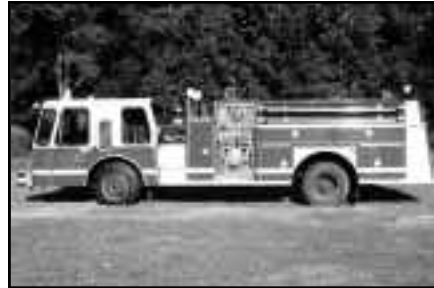
1986 E-ONE HURRICANE DIESEL/AUTOMATIC 1250 HALE / 500 GAL.
