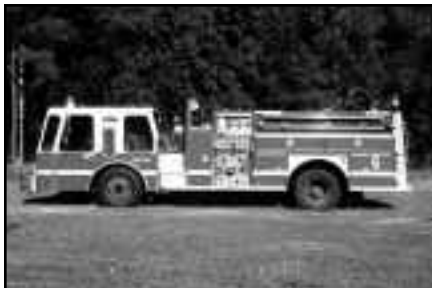
1985 E-ONE HURRICANE DIESEL/AUTOMATIC 1250 HALE / 500 GAL.
