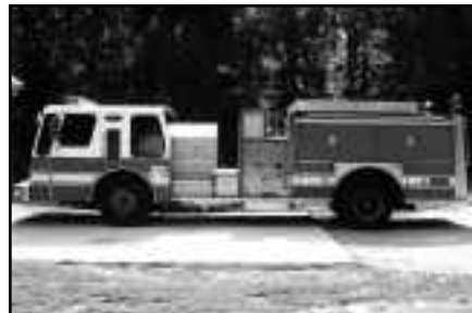
1984 E-ONE HURRICANE DIESEL/AUTOMATIC 1250 HALE / 750 GAL.
