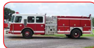
1990 E-One Cyclone Pumper Detroit 6V92TA 350 HP Diesel Allison HT-740 Automatic Hale 1500 GPM Side-Mount Pump 1000 Gallon Poly Tank Akron Foam System
