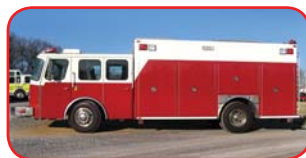
1998 E-One Heavy Rescue Cummins 8.3L 325 HP Diesel Allison MD3060P Automatic 20KW Pto Generator 12,000# Winch on Front
