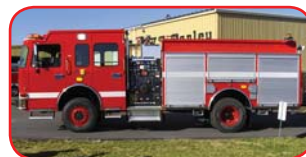
2009 Darley 4x4 Pumper/Tanker Cummins Diesel, Allison Automatic Darley 1250 GPM Pump 1250 Gallon Poly Tank PTO-Driven CAFS Compressor 30 Gallon Foam Tank
