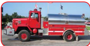
1993 Int'l 4x4 Pumper/Tanker Cummins N14 370 HP Diesel Allison HT740 Automatic Hale 1250 GPM Front-Mount Pump 1500 Gallon Stainless Steel Tank
