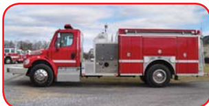
2004 FL/E-One Pumper Mercedes-Benz 300 HP Diesel Allison 3000EVS Automatic Hale 1250 GPM Top-Mount Pump 1000 Gallon Poly Tank
