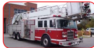
1999 Pierce Dash 110' Platform Detroit Series 60 470 HP Diesel Allison HD4060P Automatic Hale QSMG 2000 GPM Pump 300 Gallon Poly Tank FoamPro 2001 A&B Foam System
