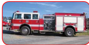
1995 Pierce Arrow 4x4 Pumper Detroit Diesel, Allison Automatic Waterous 1000 GPM PTO Pump 1000 Gallon Poly Tank Pump and Roll Capability Feecon ATP A&B Foam System
