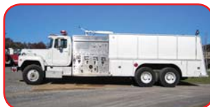
1989 Mack Foam Tanker Maxidyne 350 HP Diesel Allison Automatic Transmission Hale 2000 GPM Side-Mount Pump Feecon Foam System 2 - 1000 Gallon Foam Tanks
