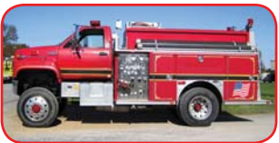
1993 GMC/E-One 4x4 Midi-Pumper Caterpillar 3116 250 HP Diesel Hale 500 GPM Side-Mount Pump 500 Gallon Poly Tank Akron 95 GPM Foam System
