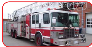
1996 HME 75' Quint Detroit Series 60 Diesel Allison Automatic Transmission Hale QSMG 2000 GPM Pump 300 Gallon Poly Tank FoamPro 2001 A&B Foam System
