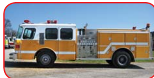
1990 E-One Hurricane Pumper Detroit 6V92TA Diesel Engine Allison Automatic Transmission Hale 1500 GPM Side-Mount Pump 500 Gallon Poly Tank
