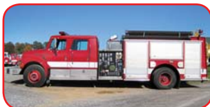
2001 Int'l/Pierce Rescue Pumper Int'l DT530 330 HP Diesel Allison Automatic Transmission Waterous 1250 GPM Pump 750 Gallon Poly Tank
