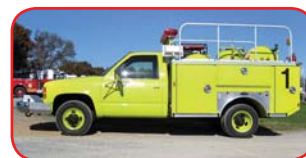
1994 4x4 ARFF Rapid Intervention Gas Engine, Automatic Transmission 50lb PKP Dry Chem System Fire Combat ARFF System 100 Gallon AFFF Water/Foam Tank
