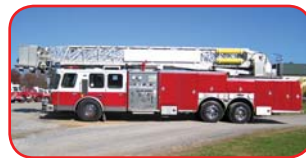
1992 E-One 95' Platform Detroit 8V92TA Diesel Engine Allison HTB741 Automatic Hale QSG125-23 1250 GPM Pump Onan 12KW Diesel Generator
