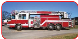
2001 Pierce Quantum 105' Quint Detroit Series 60 Diesel Allison Automatic Transmission Waterous 2000 GPM Pump 300 Gallon Poly Tank Around the Pump Foam System
