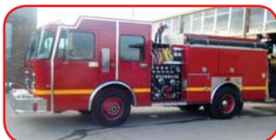
1996 Spartan/Ferrara Pumper Cummins Diesel Engine Allison Automatic Transmission Hale 1250 GPM Side-Mount Pump 1000 Gallon Poly Tank
