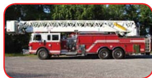
1989 Pierce Lance 105' Platform Detroit 6V92 Diesel Engine Allison Automatic Transmission Waterous 1500 GPM Pump 300 Gallon Tank
