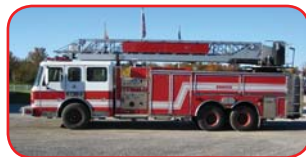
1998 American LaFrance 75' Quint Caterpillar 300 HP Diesel Allison Automatic Transmission ALF ALF150-21 1500 GPM Pump 500 Gallon Poly Tank
