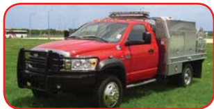
2008 Sterling 4x4 Brush Truck Cummins 305 HP Diesel Engine 6-Speed Automatic Transmission Gas-Powered CAF System 300 Gallon Polypropylene Tank 12 Gallon Foam Tank
