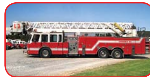
1994 Simon Duplex 105' Platform Detroit 8V92TA 475 HP Diesel Allison Automatic Transmission Waterous 2000 GPM Pump 200 Gallon Poly Tank
