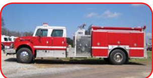
2000 Int'l/E-One Pumper Navistar 330 HP Diesel Allison Automatic Transmission Hale 1250 GPM Top-Mount Pump 1000 Gallon Poly Tank
