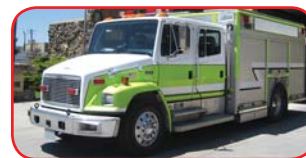
1996 FL/Becker Heavy Rescue Cummins 8.3L 300 HP Diesel Allison Automatic Transmission 35KW Generator 3-Bottle 4500psi Cascade System
