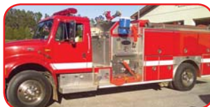
1995 Int'l/E-One Pumper Diesel Engine Allison Automatic Transmission Hale 1250 GPM Top-Mount Pump 1000 Gallon Poly Tank
