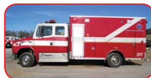
1997 E-One Ambulance/Attack Cummins 300 HP Diesel Engine Allison Automatic Transmission Hale Side-Mount PTO Pump 150 Gallon Poly Tank Robwen Foam System
