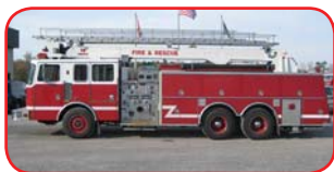
1994 KME 75' Aerial Detroit 400 HP Diesel Allison HTB741 Automatic Hale QSMG150-23 1500 GPM Pump 500 Gallon Poly Tank
