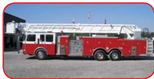
1996 Spartan/Smeal 100' Platform Detroit Series 60 470 HP Diesel Allison HD4060P Automatic Waterous CSUYBX 1500 GPM Pump 300 Gallon Poly Tank Elkhart 240-95P Foam System
