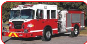
2008 Rosenbauer Rescue Pumper Caterpillar C13 485 HP Diesel Allison EVS 4000 Automatic Waterous 1500 GPM Side-Mount Pump 500 Gallon Poly Tank FoamPro 2001 Foam System
