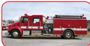
2004 Kenworth/Pierce Pumper Cummins 315 HP Diesel Allison EVS3000 Automatic Waterous 1250 GPM Side-Mount Pump 1000 Gallon Poly Tank FoamPro Foam System
