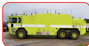
1989 Oshkosh 6x6 ARFF Vehicle Detroit 8V92TA 540 HP Diesel Hale 2000 GPM Pump 3000 Gallon Steel Tank 400 Gallon Steel Foam Tank
