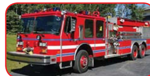
1988 E-One 6x6 Pumper/Tanker Detroit 8V92 Diesel Allison Automatic 2000 GPM Side-Mount Pump 2000 Gallon Tank
