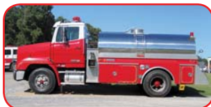
1989 FL/4-Guys Tanker Detroit Series 60 425 HP Diesel Allison HT-741 Automatic Hale Gas-Powered 200 GPM Pump 2000 Gallon Stainless Steel Tank
