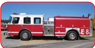
1996 E-One Cyclone Pumper Detroit 6V92TA 400 HP Diesel Allison Automatic Transmission Hale 1250 GPM Side-Mount Pump 1000 Gallon Poly Tank
