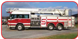
2002 Rosenbauer 75' Quint Cummins ISC 370 HP Diesel Allison Automatic Transmission Waterous CMU 1500 GPM Pump 500 Gallon Poly Tank Foam System with A & B Foam
