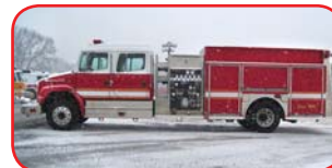
2001 FL/ALF Rescue Pumper Cat 7.2L 246 HP Diesel Allison MD3060 Automatic ALF 1250 GPM Side-Mount Pump 500 Gallon Poly Tank FoamPro Foam System
