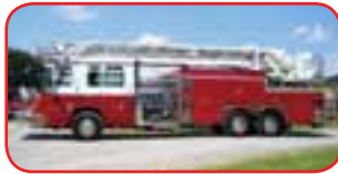
1997 Pierce Quantum 105' Quint Detroit Series 60 470 HP Diesel Allison HD 4060P Automatic Hale QSMg150-23-1500 GPM Pump 300 Gallon Poly Tank Akron 95 GPM Foam System
