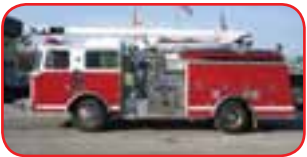
1992 KME 52' Snozzle Cummins LTA10 300 HP Diesel Allison MT-647 Automatic Hale QSG125-23 1250 GPM Pump 500 Gallon Fiberglass Tank
