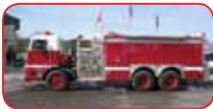
1989 AE Pumper/Tanker Detroit Series 60 425 HP Diesel Allison Hc-741 Automatic Hale QSMG 125-23 1250 GPM Pump 2000 Gallon Aluminum Tank
