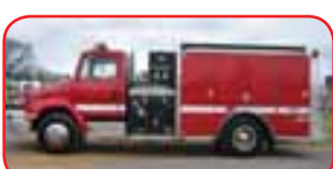
2001 ALF Commercial Pumper Cat 7.2L 300 HP Diesel Engine Allison Automatic Transmission ALF ALD-1500 1250 GPM Pump 1000 Gallon Polypropylene Tank
