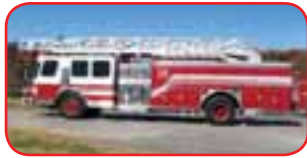
1991 E-One 75' Quint Detroit 6V92TA 400 HP Diesel Allison Automatic Hale QSMG125-23 1250 GPM Pump 500 Gallon Poly Tank Akron Foam System
