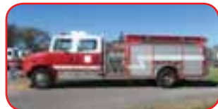
1998 FL/SC Rescue Pumper Cummins 8.3L 300 HP Diesel Allison Automatic Transmission Hale QSMG 125-23 1250 GPM Pump 500 Gallon Polypropylene Tank
