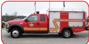
2006 Gimaex 4x4 Brush Truck Ford Power Stroke 6.4L Diesel Allison Automatic Transmission Gimaex OS-C2-110 B CAF System 250 Gallon Polypropylene Tank
