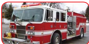
1996 Pierce Dash Rescue Pumper Detroit Series 60 Diesel Engine Allison Automatic Transmission Waterous 1500 GPM Top-Mount Pump 1000 Gallon Polypropylene Tank
