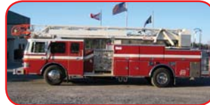
1989 Pierce Arrow 75' Quint Detroit 8V92TA Diesel Allison Automatic Transmission Waterous CSUYBX 1500 GPM Pump 300 Gallon Poly Tank
