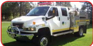
2006 GMC 4x4 Wildland Truck GMC Diesel, Allison Automatic Waterous 300GPM 300psi Diesel Pump Pump Engine: Cummins B3.3 70 HP 500 Gallon Poly Tank Foam-Pro Dual-Agent Foam System
