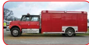
1992 Int'l/Hackney Heavy Rescue Int'l DTA466 230 HP Diesel Allison Automatic Katolight 28KW PTO Generator Ingersoll SCBA Compressor Ingersoll 4-Bottle Fill Station
