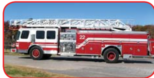
1992 E-One 75' Quint Detroit 6V92TA 400 HP Diesel Allison Automatic Hale QSMG125-23 1250 GPM Pump 500 Gallon Poly Tank Akron Foam System
