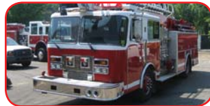
1994 KME 55' Aerial Detroit 300 HP Diesel Allison HTB741 Automatic Hale QSG125-23 1250 GPM Pump 500 Gallon Tank
