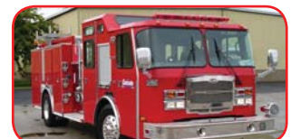
2007 E-One Rescue Pumper Cummins ISL 370 HP Diesel Allison EVS 3000 Automatic Hale QFLO 1250 GPM Top-Mount Pump 970 Gallon Poly Tank 30 Gallon Foam Tank
