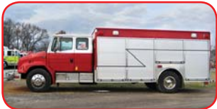
2002 FL/ALF Heavy Rescue Cummins 8.3L 315 HP Diesel Allison MD3060P Automatic Onan 25KW PTO Generator Roll-out Trays
