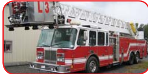
1994 Simon Duplex 95' Quint Detroit 8V92TA 475 HP Diesel Allison Automatic Transmission Waterous 2000 GPM Pump 200 Gallon Poly Tank
