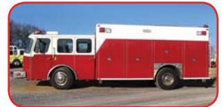
1998 E-One Heavy Rescue Cummins 8.3L 325 HP Diesel Allison MD3060P Automatic 20KW Pto Generator 12,000# Winch on Front
