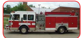
2000 Spartan Pumper/Tankers Detroit Diesel, Allison Automatic Waterous 1500 GPM Pump 1250 Gallon Poly Tank Feecon Foam System
