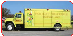
1987 Int'l/Hackney Heavy Rescue International S1900 Chassis Enclosed Seating for 3 Navistar DT466 210 HP Diesel Allison Automatic
