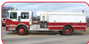
1988 Wolverine Pumper/Tanker Detroit 8V92TA Diesel Allison HT740 Automatic Hale QSMG 1500 GPM Pump 1200 Gallon Steel Tank
