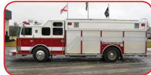
1996 Seagraves Heavy Rescue Detroit 6V92TA 400 HP Diesel Allison HT741 Automatic Winco 45KW PTO Generator Safe Air Breathing Air Compressor Four Bottle Cascade w/Refill
