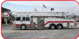
1996 Spartan/Smeal 100' Platform Detroit Series 60 470 HP Diesel Allison HD4060P Automatic Waterous CSUYBX 1500 GPM Pump 300 Gallon Poly Tank Elkhart 240-95P Foam System
