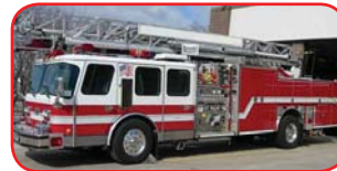
1996 E-One Hurricane 75' Quint Cummins M-11 450 HP Diesel Engine Allison Automatic Transmission Hale 1250 GPM Pump 500 Gallon Polypropylene Tank
