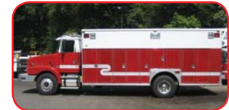
1986 American Eagle Heavy Rescue Cummins M11 330 HP Diesel Automatic Transmission Ramsey 12,000# Winch Enclosed Seating for 6
