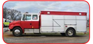
2002 FL/ALF Heavy Rescue Cummins 8.3L 315 HP Diesel Allison MD3060P Automatic Onan 25KW PTO Generator Roll-out Trays
