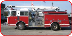
1992 KME 52' Snazle Cummins LTA10 300 HP Diesel Allison MT-647 Automatic Hale QSG125-23 1250 GPM Pump 500 Gallon Fiberglass Tank
