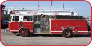
1994 KME 55' Teleboom Detroit 6V92TA 350 HP Diesel Allison HTB-741 Automatic Hale QSMG125-23 1250 GPM Pump 1250 GPM Monitor at Tip
