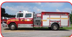
1999 FL/SC R Rescue Pumper Cummins 8.3L 300 HP Diesel Allison Automatic Transmission Hale QSG 1250 GPM Side-Mount Pump 750 Gallon Poly Tank
