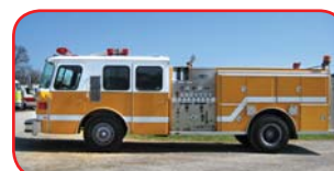
1990 E-One Hurricane Pumper Detroit 6V92TA Diesel Engine Allison Automatic Transmission Hale 1500 GPM Side-Mount Pump 500 Gallon Poly Tank
