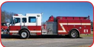
2004 ALF Custom Rescue Pumper Cummins 370 HP Diesel Allison 4000EV Automatic ALF 2000 GPM Top-Mount Pump 500 Gallon Polypropylene Tank 30 Gallon Foam Tank
