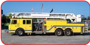
1994 Pierce Lance 105' Quint Detroit 8V92TA 500 HP Diesel Allison HD4060 Automatic Waterous CSUYBX 2000 GPM Pump 500 Gallon Poly Tank Onan 7.5KW Diesel Generator
