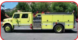
1997 Int'l/E-One Pumper Diesel, Allison Automatic Hale 1250 GPM Side-Mount Pump 1000 Gallon Polypropylene Tank
