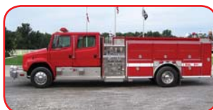
1997 FL/E-One Pumper Cummins 8.3L 325 HP Diesel Allison Automatic Transmission Hale 1250 GPM Side-Mount Pump 1000 Gallon Poly Tank Akron Foam System
