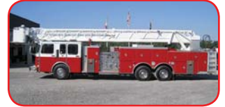
1996 Spartan/Smeal 100' Platform Detroit Series 60 470 HP Diesel Allison HD4060P Automatic Waterous CSUYBX 1500 GPM Pump 300 Gallon Poly Tank Elkhart 240-95P Foam System
