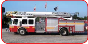
1998 E-One Hurricane 75' Quint Cummins M11 450 HP Diesel Allison HD4060P Automatic Hale QSMG150-23 1500 GPM Pump 500 Gallon Poly Tank 10KW Hydraulic Generator
