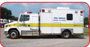
2001 FL/Medic Master Ambulance Freightliner FL-60 Chassis Enclosed Seating for 6 Cummins 5.9L 238 HP Diesel Allison Automatic Transmission Vanner 2.6KW Inverter
