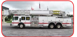
1991 E-One Hurricane 95' Platform Detroit 8V92TA 500 HP Diesel Allison Automatic Transmission Hale QSMG150 1500 GPM Pump 200 Gallon Poly Tank
