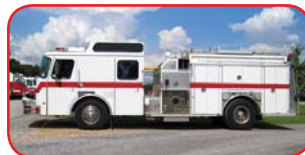
1995 E-One Custom Rescue Pumper Cummins 8.3L 300 HP Diesel Allison MD3060 Automatic Hale 1250 GPM Top-Mount Pump 1000 Gallon Polypropylene Tank FoamPro Foam System
