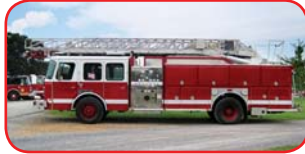
1995 E-One Cyclone 75' Quint Cummins 8.3L 300 HP Diesel Allison Automatic Transmission Hale QSG100-23 1000 GPM Pump 500 Gallon Poly Tank Akron 95 GPM Foam System
