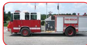
1995 Pier ce Quantum Pumper Detroit Series 60 470 HP Diesel Allison HD 4060P Automatic Waterous CMYCX 1250 GPM Pump 1000 Gallon Steel Tank
