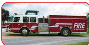
1994 E-One Hush R Rescue Pumper Detroit 6V92 400 HP Diesel Allison Automatic Transmission Hale 1250 GPM Pump w/Enclosed Panel 500 Gallon Poly Tank
