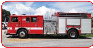
1998 Pier ce Lance Rescue Pumper Cummins M11 450 HP Diesel Allison HD4060P Automatic Waterous 1500 GPM Side-Mount Pump 750 Gallon Poly Tank Feecon ATP Foam System
