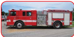
1996 Pierce Lance Rescue Pumper Cummins N14 460 HP Diesel Allison Automatic Transmission Waterous 1500 GPM Side-Mount Pump 750 Gallon Polypropylene Tank
