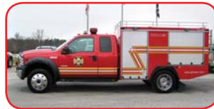
2006 Ford 4x4 Brush Truck Ford PowerStroke 6.4L Diesel Allison Automatic Transmission Gimaex OS-C2-110 B CAF System 250 Gallon Polypropylene Tank
