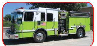
1996 HME/Becker Rescue Pumper Diesel Engine, Automatic Transmission 1500 GPM Side-Mount Pump 1000 Gallon Tank Foam Injection System
