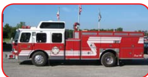
1990 E-One Hush R Rescue Pumper Detroit 6V92TA Diesel Allison Automatic Hale 1500 GPM Pump w/Enclosed Panel 500 Gallon Poly Tank
