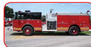
1993 Pier ce Saber Custom Pumper Detroit Series 40 Diesel Allison MD3060 Automatic Waterous 1000 GPM Top-Mount Pump 1000 Gallon Poly Tank
