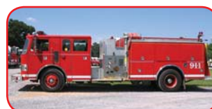
1988 Pier ce Custom Pumper Cummins M-11 350 HP Diesel Allison HT740 Automatic Waterous CMU 1500 GPM Pump 1000 Gallon Tank
