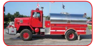
1993 International 4x4 Pumper/Tanker Cummins N14 370 HP Diesel Allison HT740 Automatic Hale 1250 GPM Front-Mount Pump 1500 Gallon Stainless Steel Tank
