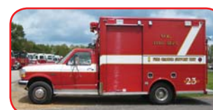
1996 Ford Service Truck Ford 7.3L Diesel Engine Allison Automatic Transmission Four-Bottle Cascade and Fill Station Honda 5KW Gas Generator
