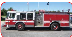
1988 E-One Hurricane Pumper Detroit 6V92TA 350 HP Diesel Allison Automatic Transmission Hale QSMG150-21 1500 GPM Pump 750 Gallon Aluminum Tank
