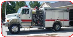
1998 Pierce 4x4 Pumper Navistar DT466 Diesel Allison MT643 Automatic Hale 2-Stage 1250 GPM Pump Pump and Roll Capability
