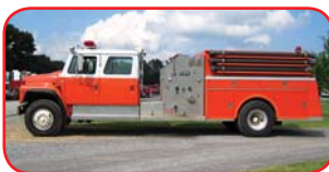
1987 Int'l/KME Pumper Navistar DT466 Diesel Engine Allison Automatic Transmission Champion 1000 GPM Top-Mount Pump 750 Gallon Steel Tank
