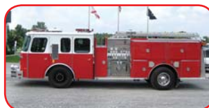
1994 E-One R Rescue Pumper Detroit 6V92TA Diesel Engine Allison Automatic Transmission Hale QSMG 1500 GPM Pump 500 Gallon Poly Tank Elkhart 240-P Foam System
