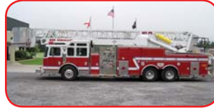
1997 KME Aerialcat 102' Platform Detroit Series 60 470 HP Diesel Allison HD4060P Automatic Hale QSMG200-23 2000 GPM Pump 150 Gallon Poly Tank
