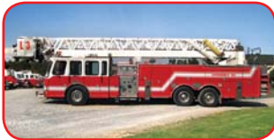
1994 Simon Duplex 95' Platform Detroit 8V92TA 475 HP Diesel Allison Automatic Transmission Waterous 2000 GPM Pump 200 Gallon Poly Tank
