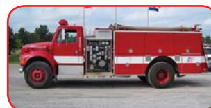
1996 Int'l/Pier ce Pumper Int'l 530 300 HP Diesel Allison Automatic Transmission Waterous 1250 GPM Side-Mount Pump 1000 Gallon Poly Tank Light Tower w/4 - 100W Lights
