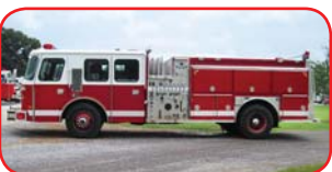
1990 E-One Cycl one Pumper Detroit 6V92TA 350 HP Diesel Allison HT-740 Automatic Hale 1500 GPM Side-Mount Pump 1000 Gallon Poly Tank
