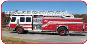
1991 E-One 75' Quint Detroit 6V92TA 400 HP Diesel Allison Automatic Hale QSMG125-23 1250 GPM Pump 500 Gallon Poly Tank Akron Foam System
