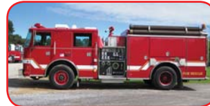
2001 Pierce Contender Pumper Detroit Series 40 330 HP Diesel Allison MD3060 Automatic Waterous CSYCX 1250 GPM Pump 1000 Gallon Poly Tank
