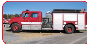
2001 Int'l Pierce Rescue Pumper Int'l DT530 330 HP Diesel Allison Automatic Transmission Waterous 1250 GPM Pump 750 Gallon Poly Tank
