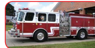
2002 E-One Cyclone II Pumper Detroit Series 60 350 HP Diesel Allison HD4060P Automatic Hale 1250 GPM Side-Mount Pump 750 Gallon Polypropylene Tank Akron Foam System
