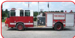
1995 Pierce Quantum Pumper Detroit Series 60 470 HP Diesel Allison HD 4060P Automatic Waterous CMYCX 1250 GPM Pump 1000 Gallon Steel Tank
