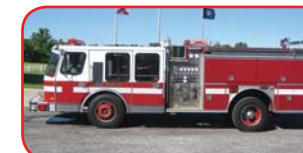
1988 E-One Hurricane Pumper Detroit 6V92TA 350 HP Diesel Allison Automatic Transmission Hale QSMG150-21 1500 GPM Pump 750 Gallon Aluminum Tank
