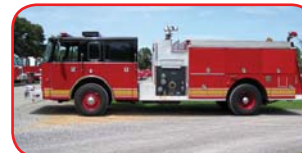
1993 Pierce Saber Custom Pumper Detroit Series 40 Diesel Allison MD3060 Automatic Waterous 1000 GPM Top-Mount Pump 1000 Gallon Poly Tank
