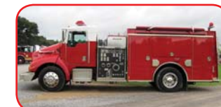
2002 Pierce Commercial Pumper Cummins ISC 325 HP Diesel Allison Automatic Transmission Waterous CSYCX 1250 GPM Pump 1000 Gallon Poly Tank
