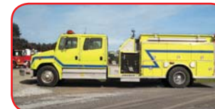
1996 FL/Southern Coach Pumper Cummins 8.3L 300 HP Diesel Allison Automatic Transmission Hale 1250 GPM Top-Mount Pump 1000 Gallon Poly Tank
