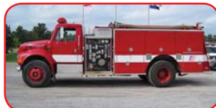
1996 Int'l/Pierce Pumper Int'l 530 300 HP Diesel Allison Automatic Transmission Waterous 1250 GPM Side-Mount Pump 1000 Gallon Poly Tank Light Tower w/4 - 100W Lights
