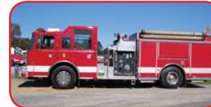
1996 Pierce Lance Pumper Detroit Series 40 320 HP Diesel Allison Automatic Transmission Waterous CSYCX 1250 GPM Pump 1000 Gallon Steel Tank Elkhart 240P Foam System
