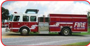
1994 E-One Hush Rescue Pumper Detroit 6V92 400 HP Diesel Allison Automatic Transmission Hale 1250 GPM Pump w/Enclosed Panel 500 Gallon Poly Tank
