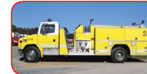
1994 FL/Firemaster Pumper Cummins ISC 300 HP Diesel Allison MD3060P Automatic Darley 1500 GPM Top-Mount Pump 1000 Gallon Poly Tank Akron Foam System
