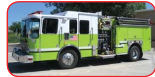
1996 HME/Becker Rescue Pumper Diesel Engine, Automatic Transmission 1500 GPM Side-Mount Pump 1000 Gallon Tank Foam Injection System
