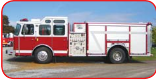
2005 E-One Rescue Pumper Cummins ISM02 400 HP Diesel Allison EVS 4000 Automatic Hale 1500 GPM Side-Mount Pump 750 Gallon Poly Tank
