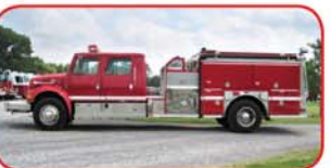
1997 Int'l/E-One Commercial Pumper Navistar DT466 Diesel Engine Allison Automatic Transmission Hale QSG 1250 GPM Top-Mount Pump 1000 Gallon Poly Tank
