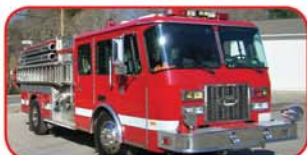
1995 E-One Sentry Pumper/Tanker Caterpillar 250 HP Diesel Allison Automatic Hale 1250 GPM Side-Mount Pump 1250 Gallon Poly Tank
