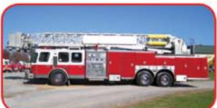
1992 E-One 95' Platform Detroit 8V92TA Diesel Engine Allison HTB741 Automatic Hale QSG125-23 1250 GPM Pump Onan 12KW Diesel Generator
