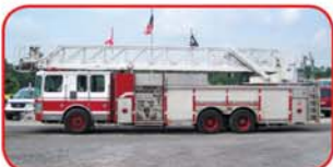
1996 HME 75' Quint Detroit Series 60 Diesel Allison HD4060P Automatic Hale QSMG200-23 2000 GPM Pump 300 Gallon Poly Tank FoamPro 2001 A&B System
