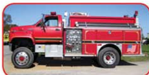
1993 GMC/E-One 4x4 Midi-Pumper Caterpillar 3116 250 HP Diesel Hale 500 GPM Side-Mount Pump 500 Gallon Poly Tank Akron 95 GPM Foam System
