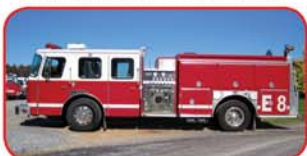
1996 E-One Cyclone Pumper Detroit 6V92TA 400 HP Diesel Allison Automatic Transmission Hale 1250 GPM Side-Mount Pump 1000 Gallon Poly Tank
