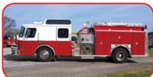
1995 E-One Rescue Pumper Cummins 8.3L 300 HP Diesel Allison MD3060 Automatic Hale 1250 GPM Top-Mount Pump 1000 Gallon Polypropylene Tank FoamPro Foam System
