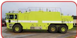
1989 Oshkosh 6x6 ARFF Vehicle Detroit 8V92TA 540 HP Diesel Hale 2000 GPM Pump 3000 Gallon Steel Tank 400 Gallon Steel Foam Tank
