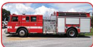
1998 Pierce Lance Rescue Pumper Cummins M11 450 HP Diesel Allison HD4060P Automatic Waterous 1500 GPM Side-Mount Pump 750 Gallon Polypropylene Tank Feecon ATP Foam System
