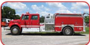
2000 Int'l/E-One Pumper Int'l 530E 300 HP Diesel Allison MD3060 Automatic Hale 1250 GPM Top-Mount Pump 1000 Gallon Poly Tank
