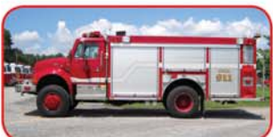
1998 Int'l/E-One 4x4 Pumper Int'l 530E 300 HP Diesel Allison MD3060P Automatic Hale CSD 1250 Pump 750 Gallon Polypropylene Tank Williams ATP-500 Foam System
