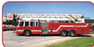
1994 Simon Duplex 95' Platform Detroit 8V92TA 475 HP Diesel Allison Automatic Transmission Waterous 2000 GPM Pump 200 Gallon Poly Tank
