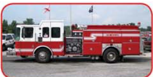
2000 HME/Ferrara Rescue Pumper Cummins 330 HP Diesel Allison MD3060 Automatic Hale QMAX 1750 GPM Pump 1000 Gallon Poly Tank Foam System with 20 Gallon Tank
