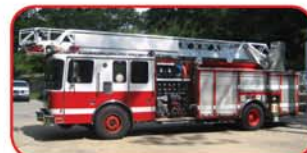
1998 HME/Ferrara 75' Quint Detroit 350 HP Diesel Allison HD4060 Automatic Darley LDM 1500 GPM Pump 300 Gallon Tank
