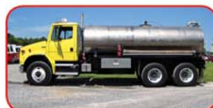
1994 FL Commercial Tanker Diesel Engine 8-Speed Manual Transmission High-Volume, Low-Pressure Pump 4000 Gallon Stainless Steel Tank
