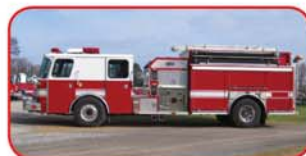
1999 E-One Rescue Pumper Cummins ISM 400 HP Diesel Allison HD4060P Automatic Hale 1250 GPM Top-Mount Pump 750 Gallon Poly Tank FoamPro System with A&B Foam
