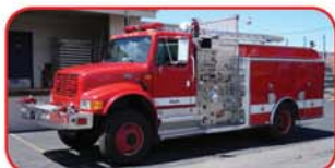
1994 Int'l 4x4 Rescue Pumper Navistar DT 466 Diesel Allison MT643 Automatic Darley 1000 GPM Auxillary Pump Cummins 6BTA-519 Pump Engine
