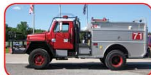
1989 Int'l 4x4 Brush Truck International DT466 Diesel Hale Auxillary-Powered Pump 500 Gallon Tank VW Diesel Pump Engine Winch on Front Bumper
