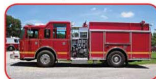
1996 Pierce Saber Custom Pumper Detroit 320 HP Diesel Allison Automatic Transmission Waterous 1250 GPM Side-Mount Pump 750 Gallon Poly Tank Akron Foam System
