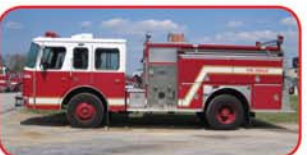
1990 E-One Protector Pumper Cummins 8.3L 250 HP Diesel Allison MT647 Automatic Hale 1000 GPM Top-Mount Pump 750 Gallon Steel Tank
