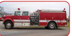
1995 Int'l/Pierce Pumper Navistar DT530 300 HP Diesel Allison Automatic Waterous 1250 GPM Side-Mount Pump 1000 Gallon Poly Tank
