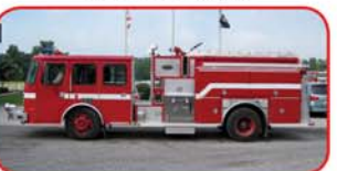
1994 E-One Cyclone Rescue Pumper Cummins 8.3L 300 HP Diesel Allison MD3060 Automatic Hale 1500 GPM Top-Mount Pump 750 Gallon Poly Tank
