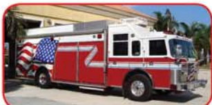
2003 Pierce Heavy Rescue/Command Cummins Diesel, Allison Automatic Onan 40KW PTO Generator Will-Burt Night Scan Light Tower Mako 6,000 psi Compressor with Fill Full-Width Command Desk
