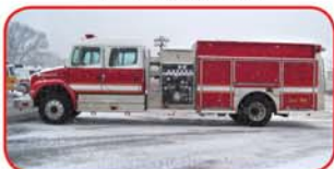
2001 FL/ALF Rescue Pumper Cat 7.2L 246 HP Diesel Engine Allison MD3060 Automatic ALF 1250 GPM Side-Mount Pump 500 Gallon Poly Tank FoamPro Foam System
