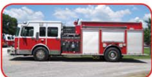
1997 Spartan Rescue Pumper Detroit Series 60 430 HP Diesel Allison Automatic Transmission Waterous 1500 GPM Side-Mount Pump 750 Gallon Polypropylene Tank A & B Foam System
