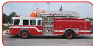
1993 E-One 50' Telesquirt Detroit 8V92 Diesel Allison Automatic Transmission Hale QSMG 2000 GPM Pump 500 Gallon Poly Tank
