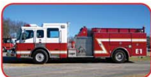
2004 ALF Rescue Pumper Cummins 370 HP Diesel Allison 4000EV Automatic ALF 2000 GPM Top-Mount Pump 500 Gallon Polypropylene Tank 30 Gallon Foam Tank
