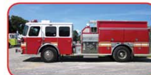
1995 E-One Protector Pumper Cummins 8.3L 350 HP Diesel Allison 3000EVS Automatic Hale 1250 GPM Top-Mount Pump 1000 Gallon Poly Tank
