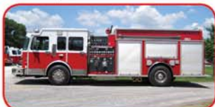
1997 Spartan Rescue Pumper Detroit Series 60 430 HP Diesel Allison Automatic Transmission Waterous 1500 GPM Side-Mount Pump 750 Gallon Polypropylene Tank A & B Foam System
