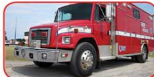
1998 FL Walk-In Heavy Rescue Cummins 300 HP Diesel Engine Allison Automatic Transmission AMPS 20KW Hydraulic Generator Cascade System
