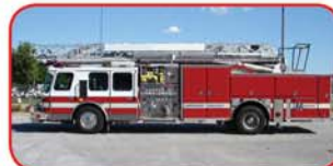
1999 E-One Hurricane 75' Quint Cummins M11 400 HP Diesel Allison HD4060 Automatic Hale QSMG 1500 Pump 500 Gallon Poly Tank Foam Educator with 30 Gallon Tank
