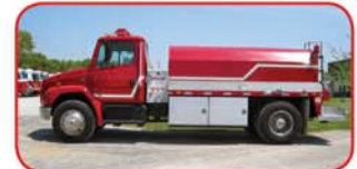
1997 FL Commercial Tanker Cummins 5.9L 210 Diesel Allison MD3060P Automatic Gorman Rupp 400 GPM Pump 1800 Gallon Stainless Steel Tank 1500 Gallon Drop Tank
