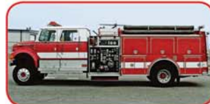
2000 Int'l/Pierce 4x4 Rescue Pumper International DT530E 330 HP Diesel Allison MD3060P Automatic Waterous 1250 GPM Side-Mount Pump 1000 Gallon Poly Tank FoamPro 1600 Foam System
