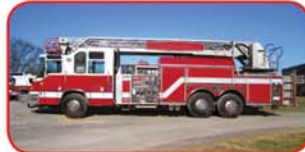
2001 Pierce Quantum 105' Quint Detroit Series 60 Diesel Allison Automatic Transmission Waterous 2000 GPM Pump 300 Gallon Poly Tank Around the Pump Foam System
