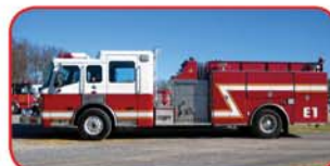
2004 ALF Rescue Pumper Cummins 370 HP Diesel Allison 4000EV Automatic ALF 2000 GPM Top-Mount Pump 500 Gallon Polypropylene Tank 30 Gallon Foam Tank
