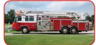
1998 Pierce Quantum 105' Quint Detroit Series 60 500 HP Diesel Allison HD4060P Automatic Waterous 2000 GPM Pump 200 Gallon Poly Tank Husky Foam System/20 Gallon Tank
