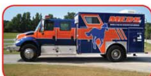
1994 International Medium Rescue Winch on Front Bumper Command Area in Rear 2 - 500W Scene Lights
