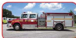
1999 FL/SC Rescue Pumper Cummins ISC 300 HP Diesel Allison MD3060 Automatic Hale 1250 GPM Side-Mount Pump 750 Gallon Poly Tank
