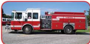
2001 HME/Ferrara Rescue Pumper Cummins 330 HP Diesel Allison MD3060 Automatic Hale QMAX 1750 GPM Pump 1000 Gallon Poly Tank Foam System with 20 Gallon Tank
