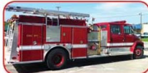
2003 FL/E-One Rescue Pumper Caterpillar 300 HP Diesel Allison EVS3000 Automatic Hale 1250 GPM Top-Mount Pump 1000 Gallon Poly Tank
