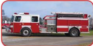
1999 E-One Rescue Pumper Cummins ISM 400 HP Diesel Allison HD4060P Automatic Hale 1250 GPM Top-Mount Pump 750 Gallon Poly Tank FoamPro System with A&B Foam
