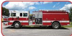
1990 Pierce Lance Rescue Pumper Detroit 6V92TA 350 HP Diesel Allison HT-740 Automatic Waterous 1500 GPM Top-Mount Pump 750 Gallon Poly Tank Feecon ATP Foam System
