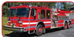
1988 E-One 6x6 Pumper/Tanker Detroit 8V92 Diesel Allison Automatic 2000 GPM Side-Mount Pump 2000 Gallon Tank
