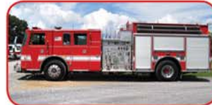
1998 Pierce Lance Rescue Pumper Cummins M11 450 HP Diesel Allison HD4060P Automatic Waterous 1500 GPM Side-Mount Pump 750 Gallon Polypropylene Tank Feecon ATP Foam System
