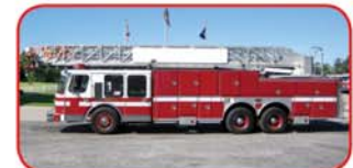
1989 Pierce Lance 105' Platform Detroit 8V92 475 HP Diesel Allison Automatic Transmission Waterous CMU 1500 GPM Pump 200 Gallon Steel Tank Onan 7.5 KW Generator
