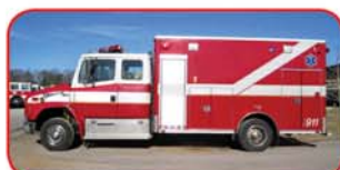
1997 E-One Ambulance/Attack Cummins 300 HP Diesel Engine Allison Automatic Transmission Hale Side-Mount PTO Pump 150 Gallon Poly Tank Robwen Foam System
