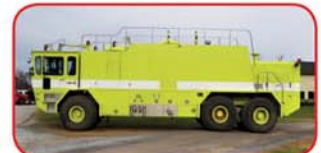
1989 Oshkosh 6x6 ARFF Vehicle Detroit 8V92TA 540 HP Diesel Hale 2000 GPM Pump 3000 Gallon Steel Tank 400 Gallon Steel Foam Tank
