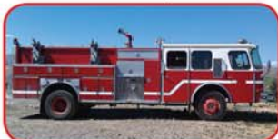
1993 E-One Cyclone 4x4 Pumper Detroit 8V92TA 450 HP Diesel Allison HT741 Automatic Hale 1500 GPM Side-Mount Pump 1000 Gallon Poly Tank
