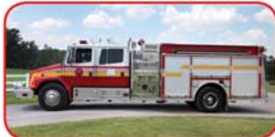
2001 FL/ALF Rescue Pumper Caterpillar 3126 300 HP Diesel Allison MD3060 Automatic Hale 1250 GPM Side-Mount Pump 750 Gallon Poly Tank
