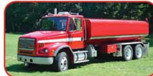
1999 Freightliner Tanker 370 Horsepower Diesel Engine Fuller Manual Transmission 600 GPM Waterous Pump 5000 Gallon Tank
