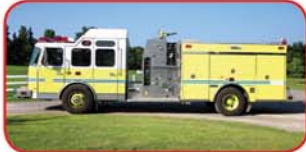
2001 E-One/Saulsbury Custom Pumper Cummins ISM 450 HP Diesel Allison HD4060 Automatic Waterous CSU 2,000 GPM Pump 1000 Gallon Poly Tank Foam System with A and B Tanks
