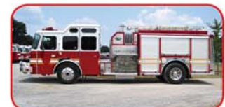
2001 E-One Typhoon Rescue Pumper Cummins ISC 350 HP Diesel Allison 3000EVS Automatic Hale 1250 GPM Side-Mount Pump 1000 Gallon Poly Tank 5KW Hydraulic Generator
