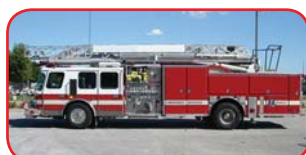
1999 E-One Hurricane 75' Quint Cummins M11 400 HP Diesel Allison HD4060 Automatic Hale QSMG 1500 Pump 500 Gallon Poly Tank Foam Eductor with 30 Gallon Tank
