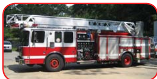
1998 HME/Ferrara 75' Quint Detroit 350 HP Diesel Allison HD4060 Automatic Darley LDM 1500 GPM Pump 300 Gallon Tank TWIN UNITS AVAILABLE!
