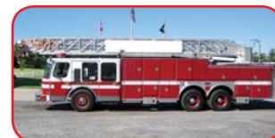
1989 Pierce Lance 105' Platform Detroit 8V92 475 HP Diesel Allison Automatic Transmission Waterous CMU 1500 GPM Pump 200 Gallon Steel Tank Onan 7.5 KW Generator
