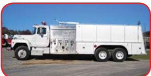
1989 Mack Foam Tanker Maxidyne 350 HP Diesel Allison Automatic Transmission Hale 2000 GPM Side-Mount Pump Feecon Foam System 2 - 1000 Gallon Foam Tanks
