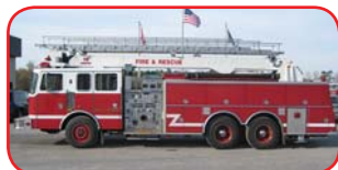
1994 KME 75' Aerial Detroit 400 HP Diesel Allison HTB741 Automatic Hale QSMG150-23 1500 GPM Pump 500 Gallon Poly Tank
