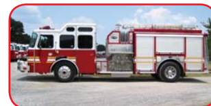
2001 E-One Typhoon Rescue Pumper Cummins ISC 350 HP Diesel Allison 3000EVS Automatic Hale 1250 GPM Side-Mount Pump 1000 Gallon Poly Tank 5KW Hydraulic Generator
