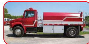
1997 FL Commercial Tanker Cummins 5.9L 210 Diesel Allison MD3060P Automatic Gorman Rupp 400 GPM Pump 1800 Gallon Stainless Steel Tank 1500 Gallon Drop Tank
