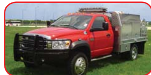
2008 Sterling 4 x 4 Brush Truck Cummins 305 HP Diesel Engine 6-Speed Automatic Transmission Gas-Powered CAF System 300 Gallon Polypropylene Tank 12 Gallon Foam Tank
