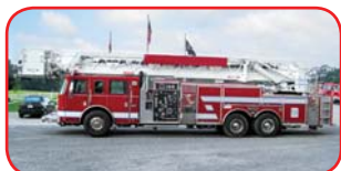
2002 Pierce Dash 100' Platform Detroit Series 60 500 HP Diesel Allison HD4060P Automatic Waterous CMU 2000 GPM Pump 500 Gallon Poly Tank
