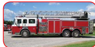
1998 American LaFrance 75' Quint Caterpillar 300 HP Diesel Allison Automatic Transmission ALF ALF150-21 1500 GPM Pump 500 Gallon Poly Tank
