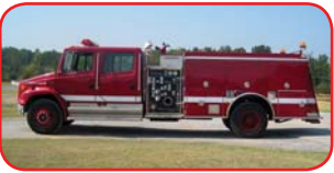
1996 FL/Pierce Commercial Pumper Cummins 8.3L 300 HP Diesel Allison MD3060P Automatic Waterous 1250 GPM Pump 1000 Gallon Poly Tank Piped for Deck Gun
