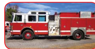
1992 Simon Duplex/Saulsbury Pumper Detroit 8V92 450 HP Diesel Allison HT740 Automatic Hale QSMG175-23S 1750 GPM Pump 1200 Gallon Fiberglass Tank Akron Apollo Deck Gun with TFT Tip
