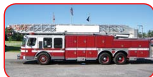
1989 E-One Hurricane 110' Aerial Detroit 8V92TA 475 HP Diesel Allison Automatic Onan 6KW Diesel Generator Akron Gemini Monitor at Tip
