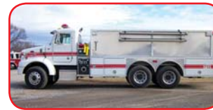
2003 Peterbilt Pumper/Tanker Caterpillar 3126E 330 HP Diesel Allison MD3060P Automatic Waterous 750 GPM Pump 2500 Gallon Poly Tank
