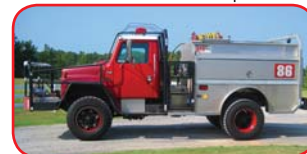
1989 Int'l/Southern Coach 4x4 Brush Truck International B170F 170 HP Diesel Allison MT643 Automatic Hale Auxillary 400 GPM Pump 500 Gallon Fiberglass Tank
