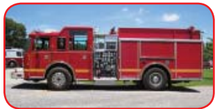
1996 Pierce Saber Custom Pumper Detroit 320 HP Diesel Allison MD3060 Automatic Waterous 1250 GPM Side-Mount Pump 750 Gallon Poly Tank Akron Foam System
