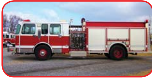
1997 Spartan/Southern Coach Pumper Cummins C8.3 325 HP Diesel Allison MD3060 Automatic Hale 1500 GPM Pump 750 Gallon Poly Tank Foam Poly Tank
