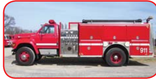
1998 Ford/E-One Pumper Cummins 8.3L 250 HP Diesel Allison MD3060P Automatic Hale 1250 GPM Pump 1000 Gallon Poly Tank Piped for Deck Gun
