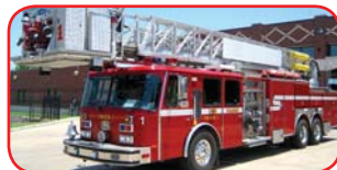
1994 E-One Hurricane 95' Platform Detroit 8V92 450 HP Diesel Allison HT740 Automatic Waterous 2000 GPM Pump 200 Gallon Poly Tank Foam System with 20 Gallon Foam Cell
