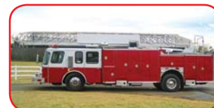
1995 E-One 110' Ladder Detroit 6V92TA Diesel Allison HT 740 Automatic Fabco Power 8KW PTO-Drive Generator Seating for 7 - 4 SCBA Seats
