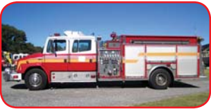
1999 FL Southern Coach Pumper Cummins 8.3L HP Diesel Allison MD3060P Automatic Hale QSG125-23 1250 GPM Pump 750 Gallon Poly Tank Honda 3.5KW Gas Generator
