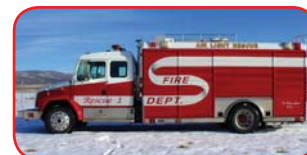
2000 FL/Hackney Heavy Rescue Cummins ISC 330 HP Diesel Allison 3000 EVS Automatic Onan 40KW 3 Phase Generator Telescoping Mast with Auto Stow Scott 5000 PSI SCBA Compressor
