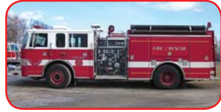
1997 Pierce Saber Custom Pumper Detroit Series 40 330 HP Diesel Allison MD3060P Automatic Waterous 1500 GPM Pump 750 Gallon Poly Tank Apollo/Akron Deck Gun
