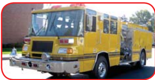
1996 Pierce Quantum Pumper Detroit Diesel Allison Automatic Hale 1500 GPM Pump 750 Gallon Poly Tank
