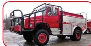
1994 FL 4x4 Brush Truck 170 HP Diesel Allison MT643 Automatic Hale Auxillary 400 GPM Pump 650 Gallon Poly Tank
