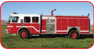
1993 E-One Cyclone 4x4 Pumper Detroit 8V92TA 450 HP Diesel Allison HT741 Automatic Hale 1500 GPM Pump 1000 Gallon Poly Tank Piped for Deck Gun
