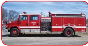
1995 Freightliner Darley Pumper Cummins 8.3L 300 HP Diesel Allison MD3060P Automatic Darley 1500 GPM Pump 750 Gallon Galvanized Tank TFT Crossfire Deck Gun
