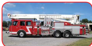
2002 E-One 100' Bronto Platform Cummins ISM 500 HP Diesel Allison HD4560P Automatic Waterous S100C10D 2000 GPM Pump 250 Gallon Poly Tank
