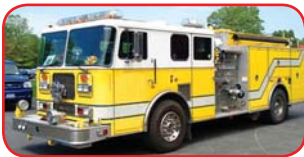
1997 Seagrave Custom Pumper Waterous 1500 GPM Pump 500 Gallon Tank 5KW Diesel Generator
