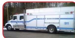
2003 Pierce/Kenworth Heavy Rescue 21' Rescue Body Harrison Hydraulic Generator On-Board 4-Bottle Cascade Refrigerator
