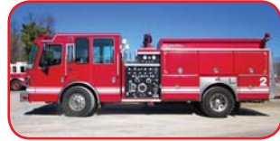
2000 Ferrara Inferno Pumper Cummins 400 HP Diesel Allison HD4060 Automatic Hale 1250 GPM Pump 1000 Gallon Poly Tank Apollo/Akron Deck Gun
