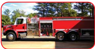
2007 FL/ALF Pumper/Tanker Caterpillar C9 Diesel Allison MD3060 Automatic Hale 1250 GPM Pump 3000 Gallon Drop Tank 2500 Gallon Poly Tank
