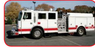
1990 Simon Duplex/Saulsbury Pumper Detroit 6V-92 350 HP Diesel Allison Automatic Hale 1750 GPM Pump 750 Gallon Tank Harrison 15KW Diesel Generator
