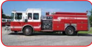
2001 HME/Ferrara Rescue Pumper Cummins 330 HP Diesel Allison MD3060 Automatic Hale QMAX 1750 GPM Pump 1000 Gallon Poly Tank Foam System with 20 Gallon Tank
