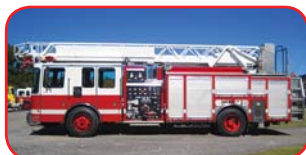
1998 HME/Ferrara 75' Quint Detroit Series 60 350 HP Diesel Allison HD4060 Automatic Darley LDM 1500 GPM Pump 300 Gallon Tank
