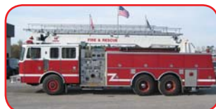
1994 KME 75' Firestix Aerial Detroit 400 HP Diesel Allison HTB741 Automatic Hale QSMG150-23 1500 GPM Pump 500 Gallon Poly Tank
