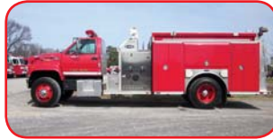
2001 GMC/E-One Commercial Pumper Caterpillar 3126 246HP Diesel Allison MD3060 Automatic Hale 1250 GPM Pump 1000 Gallon Poly Tank Honda 5KW Gas Generator
