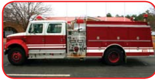
1991 Int'l/KME Commercial Pumper Navistar Int. DTA466 E245 HP Engine Allison Transmission Hale 1250 GPM Pump 1000 Gallon Fiberglass Tank
