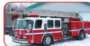
1992 E-One Hurricane 75' Quint Detroit 8V-92TA 450 HP Diesel Allison Automatic Hale 1500 GPM Pump 400 Gallon Poly Tank Prepiped Monitor
