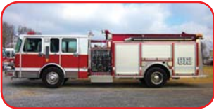
1997 Spartan/Southern Coach Pumper Cummins C8.3 325 HP Diesel Allison MD3060 Automatic Hale 1500 GPM Pump 750 Gallon Poly Tank Foam Poly Tank
