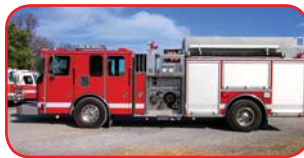
1993 HME/Quality Rescue Pumper Detroit 6V92 400 HP Diesel Allison HT740 Automatic Waterous 1750 GPM Pump 500 Gallon Poly Tank Elkhart Deck Gun
