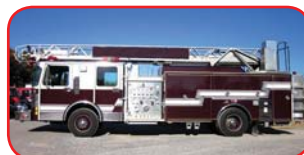
1997 Ferrara Spartan RK 60' Ladder Cummins 325 HP Diesel Allison MD306P Automatic Hale QSMG175-17L 1750 GPM Pump 500 Gallon Poly Tank
