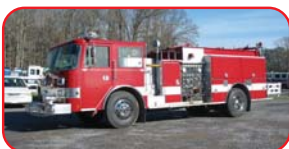
$79,000 1990 Pierce Arrow Custom Pumper 1250 Waterous Side Mount Pump 750 Gallon Steel Tank Allison Automatic Detroit Diesel
