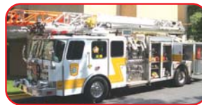
Call for Pricing 1998 E-One 75' Quint 1500 Hale Side Mount Pump 500 Gallon Poly Tank 30 Gallon Akron Foam Tank Detroit Diesel
