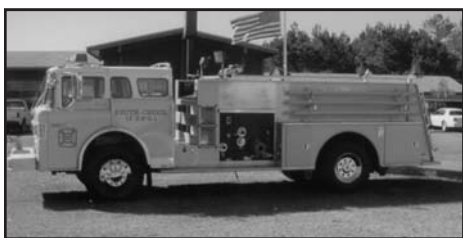
1982 Seagrave Diesel 1500 GPM Waterous
