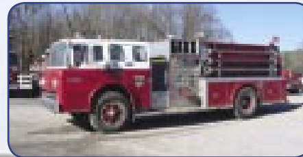
$35,000 1982 Sanford Pumper Ford C-8000 Chassis 1000 Hale Side Mount Pump 1100 Gallon Steel Tank Diesel Engine/ Automatic
