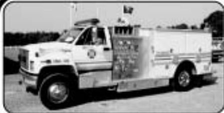
$74,000 1994 Chevy Kodiak 1250 Hale Side Mount Pump 500 Gallon Poly Tank Cat Diesel/ Allison Automatic Add $6K for 950 Gallon Tank
