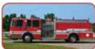
1996 Spartan Rescue Pumper Detroit Series 60-470 HP Diesel Allison Automatic Waterous 1500 GPM Side-Mount Pump 750 Gallon Poly Tank 6000W Folding Light Tower
