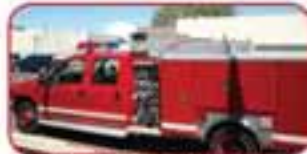
2003 Ferrara 4x4 F-550 Mini Pumper 500 GPM CPS Pump 300 Gallon Booster Tank Pump and Roll Capability 12,000# Winch
