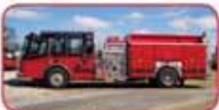
2001 Ferrara Inferno Rescue Pumper Detroit Series 60, Allison MD4560 Hale QMAX 1250 GPM Side-Mount Pump 500 Gallon Poly Tank Interior Medical Cabinet TWIN UNITS AVAILABLE!
