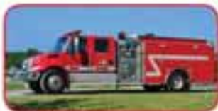
2005 Smeal / Int'l Rescue Pumper Int'l Diesel, Allison Automatic Waterous 1500 GPM Side-Mount Pump 1000 Gallon Poly Tank 5000W Generator
