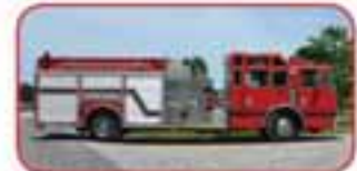
2002 KME Panther Rescue Pumper Detroit Series 50, Allison MD3060P Hale QMAX 1500 GPM Top-Mount Pump Foam Pro 2001 A & B System 750 Gallon Poly Tank 10KW Hydraulic Generator
