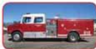
1997 Custom / Freightliner Pumper Detroit Series 55 Diesel Allison Automatic Transmission Waterous 1500 GPM Side-Mount Pump 500 Gallon Poly Tank
