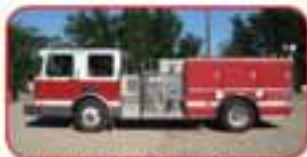
1992 Quality / Spartan Pumper Detroit 6V92TA, Allison HT740 Waterous 1250 GPM Side-Mount Pump 500 Gallon Fiberglass Tank Feecon ATP Foam System 50 Gallon Foam Tank
