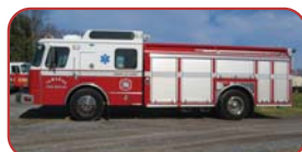
1997 E-One Hush Rescue Pumper/EMSTransport Unit Cummins Diesel, Allison Automatic Hale 1250 GPM Rear Mount Pump 500 Gallon Poly Tank
