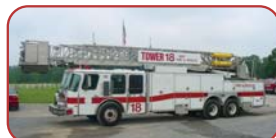
1986 E-One 95' Tower Detroit 8V92TA 475 HP Diesel Allison Automatic Transmission 12,000 Watt Diesel Generator
