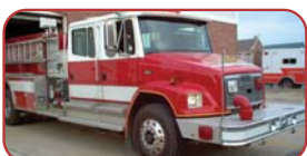
1994 Ferrara/FL80 Pumper Cummins 8.3L Diesel Engine Allison Automatic Transmission 1250 GPM Side Mount Pump 1000 Gallon Poly Tank
