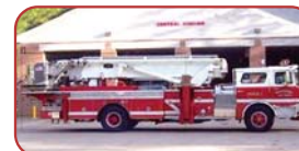
1973 Mack 75' Baker Aerialscope Retired FDNY Ladder 79 Thermodyne 260 HP Diesel Allison MT 647 Automatic
