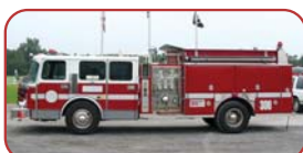
1991 Southern Coach Pumper Cummins 300 HP Diesel Allison HT740 Automatic American Godiva 1500 GPM Pump 750 Gallon Poly Tank
