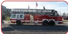
1991 E-One 95' Platform Detroit 8V92TA 450HP Diesel Allison HTB741 Automatic American Godiva 1500 GPM Pump 200 Gallon Poly Tank
