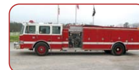
1989 Pierce Arrow Rescue Pumper Detroit 8V92TA 475 HP Diesel Allison HT740 Automatic Waterous 2-Stage 1500 GPM Pump 500 Gallon Poly Tank
