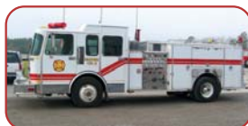
1994 E-One/Spartan Pumper Cummins 300 HP Diesel Engine Allison MD3060P Automatic Hale 1250 GPM Side Mount Pump 500 Gallon Poly Tank
