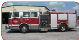
1988 American Eagle/ Spartan Pumper Detroit Diesel, Allison Automatic Hale 1750 GPM Pump 750 Gallon Poly Tank
