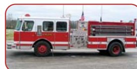
1989 E-One Hurricane Pumper Detroit 6V92TA Diesel Allison HT740 Automatic Hale 1250 GPM Side Mount Pump 1000 Gallon Poly Tank
