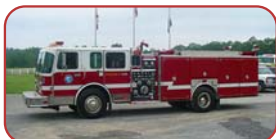
1993 Ferrara Silent Knight Custom Pumper Cummins Diesel, Allison Automatic Hale 1250 GPM Pump 500 Gallon Poly Tank
