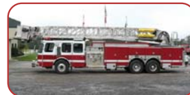
1995 E-One 95' Platform Detroit 8V92TA Diesel Engine Allison Automatic Transmission Hale 1500 GPM Side Mount Pump 300 Gallon Polypropylene Tank
