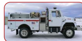
1980 WS/Int'l 4x4 Quick Attack Ford Gas Engine, Int'l Automatic AccuFoam Foam System Waterous 350 GPM Side Mount Pump 500 Gallon Steel Coated Tank
