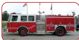
1997 E-One Cyclone II Pumper Detroit Series 40 330 HP Diesel Allison Automatic Transmission Hale 1250 GPM Side Mount Pump 500 Gallon Poly Tank
