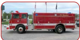
1991 Pierce Dash Heavy Rescue Caterpillar 3208T 250 HP Diesel Allison MT643 Automatic 4 - 1500W Quartz Lights Piped for Deck Gun
