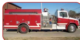
1999 KME FL80 Pumper Cummins 330 HP Diesel Allison Automatic Transmission Hale 1500 GPM Pump 1000 Gallon Poly Tank
