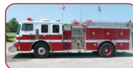
1983 E-One Custom Pumper Detroit 8V92TA 370 HP Diesel Allison Automatic Transmission Hale 1250 GPM Side Mount Pump 1000 Gallon Aluminum Tank
