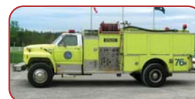
1985 Ford/EEI Tanker Caterpillar 210 HP Diesel Engine Allison MT643 Automatic Hale 250 GPM Side-Mount Pump 1500 Gallon Steel Tank
