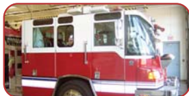
1996 Pierce Quantum Rescue Pumper Detroit Diesel, Allison Automatic Waterous 1250 GPM Pump 750 Gallon Poly Tank
