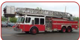
1988 E-One 95' Platform Detroit 8V92TA 475HP Diesel Allison HT740 Automatic Hale 1500 GPM Side Mount Pump 300 Gallon Aluminum Tank
