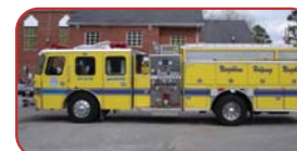
1990 E-One Rescue Pumper Detroit 8V92 Diesel Engine Allison HT740 Automatic 1500 GPM Side Mount Pump 500 Gallon Poly Tank
