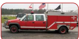
1998 GMC/E-One 4x4 Brush Truck Chevy 6.5L Diesel Turbo Engine Automatic Transmission Berkeley 200 GPM Pump 250 Gallon Poly Tank
