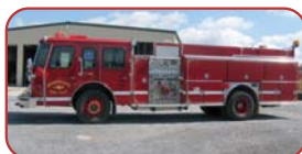
1989 E-One Hush Pumper Detroit 6V92TA Diesel Allison HTD741 Automatic Hale 1500 GPM Pump 750 Gallon Aluminum Tank
