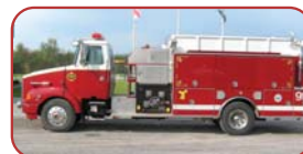
1992 Beck/Volvo Pumper Tanker Detroit 60 Series 350 HP Diesel Allison HT740 Automatic Hale QSG 1500 GPM Pump 1500 Gallon Poly Tank
