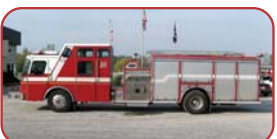
1997 E-One Cyclone Hush Pumper Detroit Diesel, Allison Automatic Interior Command Desk Hale 1500 GPM Pump 500 Gallon Tank
