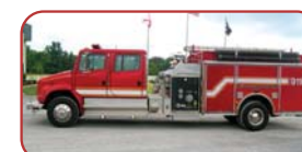
1997 Pierce/FL Rescue Pumper Cummins 8.3L Diesel Allison Automatic Transmission Waterous 1500 GPM Pump 1000 Gallon Poly Tank
