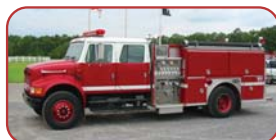
1992 E-One/FL Pumper Int'l 250 HP Diesel Engine Allison Automatic Transmission Hale 1250 GPM Side Mount Pump 500 Gallon Poly Tank
