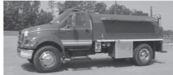
2005 FORD F750 - CAT DIESEL - AUTO A/C - 1850 STAINLESS TANK - EM LIGHTS 500 PUMP - SUCTION HOSE - 2 COMPS
