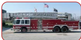
1992 E-One 95' Platform Detroit 8V92 Diesel Engine Allison Automatic Transmission Godiva 1500 GPM Pump 200 Gallon Tank
