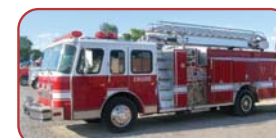
1989 Hush 50' Telesqurt Detroit 6V92TA Diesel Engine Allison Automatic Transmission Hale 1250 GPM Pump 500 Gallon Poly Tank
