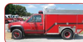
1998 E-One/AE 4x4 Quick Attack GM 6.5L 195 HP Diesel Engine Automatic Transmission Berkley 250 GPM Skid Unit 300 Gallon Poly Tank
