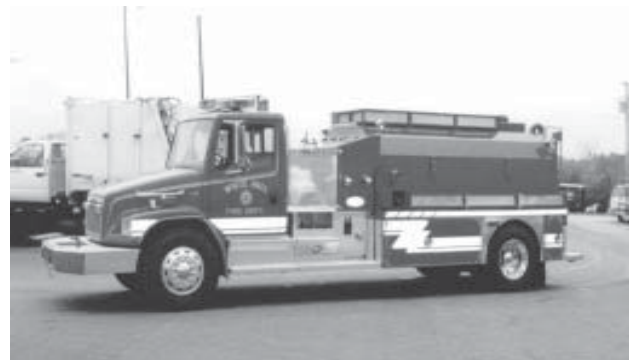
2005 FORD F750 - CAT DIESEL - AUTO A/C - 1850 STAINLESS TANK - EM LIGHTS 500 PUMP - SUCTION HOSE - 2 COMPS
