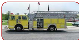
1991 Sutphen 75' Quint Detroit Diesel, Allison Automatic Hale 1500 GPM Side Mount Pump 400 Gallon Fiberglass Tank Rockwell Foam System
