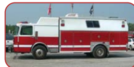
1996 Saulsbury Heavy Rescue Spartan Chassis Cummins Diesel, Allison Automatic Harrison 1500 Watt Generator 5 Quartz Lights, 2 Scene Lights
