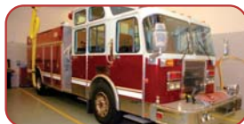
1991 Spartan Rescue Pumper Diesel Engine, Automatic Transmission Top Mount Enclosed Pump 750 Gallon Poly Tank
