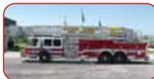
1990 E-One 95' Platform Detroit 8V92TA Diesel Allison HT-740 Automatic Hale QSMG150-21 1500 GPM Pump 200 Gallon Poly Tank
