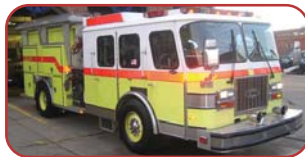
1993 E-One Rescue Pumper Detroit 450 HP Diesel Allison HT 740 Automatic Hale 2000 GPM Side-Mount Pump 750 Gallon Poly Tank Williams Foam System
