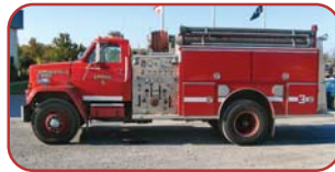
1987 E-One Commercial Pumper Detroit 6V71 Diesel Engine Allison Automatic Transmission Hale 1000 GPM Side-Mount Pump 1000 Gallon Poly Tank
