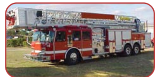
2002 E-One 105' Platform Cummins ISM 500 HP Diesel Allison HD4060P Automatic Hale 1500 GPM Side Mount Pump 150 Gallon Poly Tank Akron Dual Monitors at Tip
