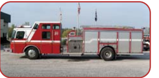
1997 E-One Hush Rescue Pumper Detroit Diesel, Allison Automatic Interior Command Desk Hale 1500 GPM Pump 500 Gallon Tank
