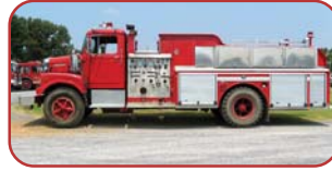
1969 White/Trautweins Pumper Cummins Diesel, CumFuller Automatic Hale 1250 GPM 2-Stage Pump Robwen Model 500 Foam System 600 Gallon Poly Tank
