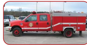
2000 ALF 4x4 Quick Attack Ford Diesel, Automatic Transmission Independently Diesel Powered Pump 250 Gallon Poly Tank FoamPro System
