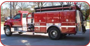
1993 Ferrara Pumper/Tanker Diesel Engine Automatic Transmission 1250 Top-Mount Pump 1250 Gallon Tank
