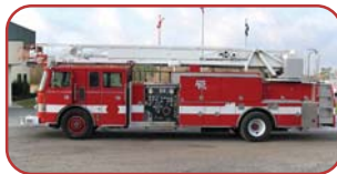
1990 Pierce Lance 75' Quint Cummins 400 HP Diesel Engine Allison HT-740 Automatic Waterous 1500 GPM Pump 300 Gallon Steel Tank
