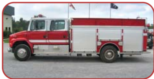
1998 Clay Fire/FL Rescue Pumper Cummins 8.3L 325 HP Diesel Allison Automatic Hale 1500 GPM Rear-Mount Pump 750 Gallon Poly Tank
