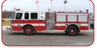
1990 E-One Protector Pumper Cummins Diesel Engine Allison Automatic Hale QSG 1250 GPM Pump 500 Gallon Poly Tank
