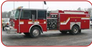
1994 Ferrara Pumper Cat 3116 300 HP Diesel Allison Automatic Hale 1250 GPM Pump 1000 Gallon Poly Tank
