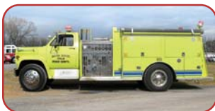
1987 GMC/FMC Pumper Detroit 8.2L Turbo Diesel Clark 557 5-Speed Manual Hale 1000 GPM Pump 1000 Gallon Steel Tank
