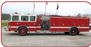
1989 Pierce Arrow Rescue Pumper Detroit 8V92TA 475 HP Diesel Allison HT740 Automatic Waterous 2-Stage 1500 GPM Pump 500 Gallon Poly Tank
