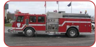
1989 E-One Hurricane Rescue Pumper Detroit 8V92 445 HP Diesel Allison HT-740 Automatic Hale 1500 GPM Side-Mount Pump 500 Gallon Poly Tank
