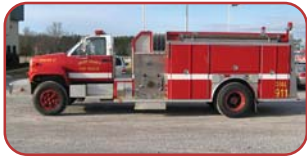
2002 ALF Rescue Pumper Caterpillar 3116 250 HP Diesel Automatic Transmission Hale 1250 GPM Top-Mount Pump 1000 Gallon Poly Tank
