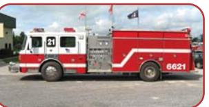
2001 ALF Rescue Pumper Detroit Diesel, Allison Automatic ALF 2000 GPM Side-Mount Pump Elkhart 125 GPM Foam System 750 Gallon Poly Tank
