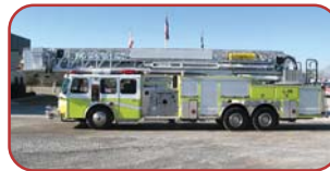
2002 E-One 105' Platform Cummins ISM 500 HP Diesel Allison HD4060P Automatic Hale 1500 GPM Side Mount Pump 150 Gallon Poly Tank Akron Dual Monitors at Tip
