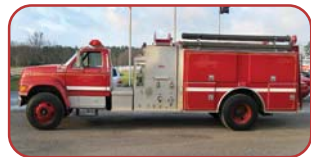
1997 Ford Commercial Pumper Cummins 8.3L 250 HP Diesel Eaton 5-Speed Manual Hale 1000 GPM Top-Mount Pump 1000 Gallon Poly Tank
