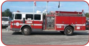
1991 Southern Coach Pumper Cummins LTA10 300 HP Diesel Allison HT740 Automatic American Godiva 1500 GPM Pump 660 Gallon Poly Tank
