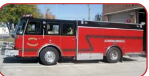
2002 Saulsbury Rescue Pumper Cummins Diesel, Allison Automatic Hale 1500 GPM Rear Mount Pump 500 Gallon Poly Tank Foam Pro Injection System
