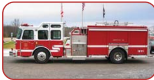
2003 E-One Rescue Pumper Cummins Diesel, Allison Automatic Hale 1500 GPM Top-Mount Pump FoamPro System, 20 Gallon Foam Tank 1000 Gallon Poly Tank
