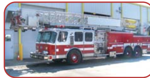
1990 E-One 95' Platform Diesel Engine Automatic Transmission Hale 1500 GPM Side Mount Pump 200 Gallon Poly Tank
