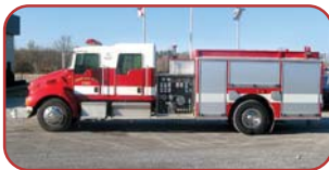
2004 Pierce/Kenworth Pumper Cummins 8.3L 315 HP Diesel Allison Automatic Waterous CSYCX 1250 Pump 1000 Gallon Poly Tank
