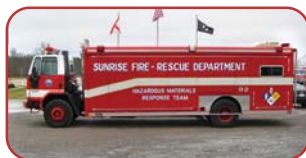
1989 Ford/Hackney Heavy Rescue/Hazmat Interior Command Center in Rear Ford Diesel, Allison Automatic Onan 7.5KW Hydraulic Generator Light Tower with 2 -1500W Lights
