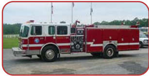
1993 Ferrara Silent Knight Pumper Cummins 320 HP Diesel Engine Allison Automatic Transmission Hale 1250 GPM Side Mount Pump 500 Gallon Poly Tank
