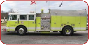
1993 Pierce Rescue Pumper Detroit 6492TA 350 HP Diesel Allison HT 740 Automatic Waterous 1500 GPM Pump 750 Gallon Steel Tank Elkhart Foam System
