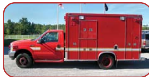
2003 Ford/Taylor Made Ambulance Ford F-450 Chassis Taylor Made Type I Ambulance Body Ford 7.3L Diesel Engine Ford Automatic Transmission
