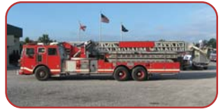
1993 Sutphen 100' Platform Cummins 410 HP Diesel Engine Allison Automatic Transmission 2 Monitors at Tip
