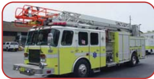
2000 E-One HP 75' Quint Cummins ISM 400 HP Diesel Allison HD 4060P Automatic Hale 1000 GPM Pump 500 Gallon Poly Tank
