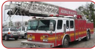
1995 E-One 110' Ladder Detroit 6V92TA Diesel Allison HT 740 Automatic Piped Waterway 8KW PTO-Driven Generator
