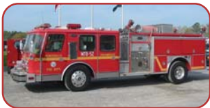
1990 E-One Hurricane Pumper Detroit 8V92 450 HP Diesel Allison HT741 Automatic Hale 1500 GPM Top Mount Pump 500 Gallon Poly Tank
