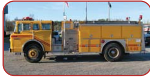
1988 Ford/E-One Pumper Caterpillar 3208 Diesel Engine Allison MT-643 Automatic Hale 1250 GPM Top-Mount Pump 1000 Gallon Poly Tank
