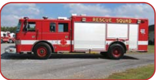
1992 Pierce Lance Heavy Rescue Cummins 350 HP Diesel Engine Allison HT740 Automatic Light Tower, PTO Generator 12,000Lb Winch
