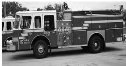
$75,500 1986 E-One Hush 1250 Hale Pump 750 Fiberglass Tank Detroit 6-71 Diesel Allison Automatic
