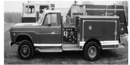
$8,000 1975 Pierce Mini-Pumper 400 GPM Waterous 200 Gallon Steel Tank Gas 4-speed
