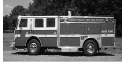
$99,000 1988 Saulsbury Heavy Rescue 250 Pump/200 Gal Water Winch, Generator, Cascade Detroit 6V-92TA Diesel Allison Automatic
