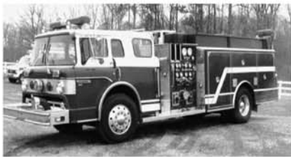
$65,000 1988 Ward Rescue Pumper 1250 Hale Pump 750 Poly Tank Caterpillar 3208 Diesel Automatic
