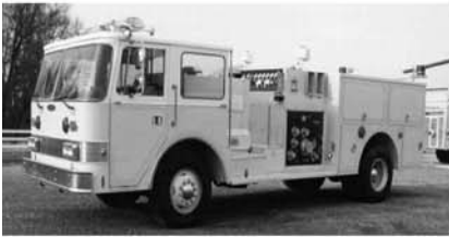
$45,000 1984 Pierce Arrow 1500 Waterous Pump 750 Gallon Tank Detroit 6V92TA Diesel Allison Automatic
