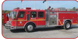
1990 E-One Hurricane Pumper Detroit 8V92 450 HP Diesel Allison HT741 Automatic Hale 1500 GPM Top Mount Pump 500 Gallon Poly Tank
