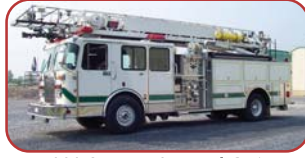
1989 Spartan/LTI 75' Quint Cummins Diesel Engine Waterous 1500 GPM Pump 300 Gallon Tank 7,500 Watt Onan Generator
