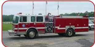
1993 Ferrara Silent Knight Pumper Cummins 320 HP Diesel Engine Allison Automatic Transmission Hale 1250 GPM Side Mount Pump 500 Gallon Poly Tank
