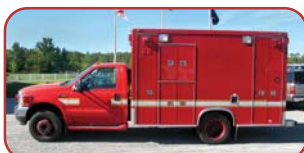
003 Ford/Taylor Made Ambulance Ford F-450 Chassis Taylor Made Type I Ambulance Body Ford 7.3L Diesel Engine Ford Automatic Transmission
