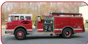
1980 Ford C-8000 Pumper Caterpillar 3208 Diesel Engine Allison Automatic Transmission 1250 GPM Pump 750 Gallon Tank
