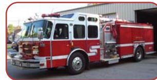
2003 E-One Rescue Pumper Cummins ISC 350 HP Diesel Allison MD 3066P Automatic Hale 1500 GPM Top-Mount Pump FoamPro System, 20 Gallon Foam Tank 1000 Gallon Poly Tank
