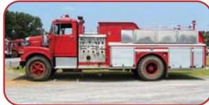
1969 White/Trautweins Pumper Cummins Diesel, CumFuller Automatic Hale 1250 GPM 2-Stage Pump Robwen Model 500 Foam System 600 Gallon Poly Tank
