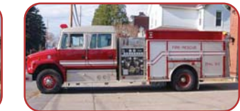
2002 ALF Rescue Pumper Cummins ISC 330 HP Diesel Allison MD3060P Automatic Hale 1500 GPM Side Mount Pump 750 Gallon Polypropylene Tank
