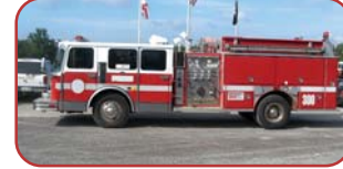
1991 Southern Coach Pumper Cummins LTA10 300 HP Diesel Allison HT740 Automatic American Godiva 1500 GPM Pump 660 Gallon Poly Tank
