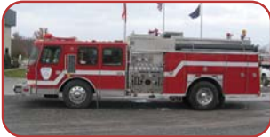
1989 E-One Rescue Pumper Detroit 8V92 445 HP Diesel Allison HT-740 Automatic Hale 1500 GPM Side-Mount Pump 500 Gallon Poly Tank
