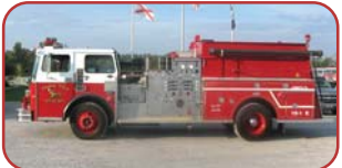
1982 Pirsch/Spartan Pumper Detroit 8V71 316 HP Diesel Allison Automatic Transmission Hale 1500 GPM Side-Mount Pump 1000 Gallon Poly Tank
