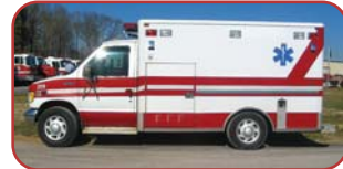
1993 NAB Type III Ambulance Ford E-350 Chassis International 7.3L Turbo Diesel Ford Automatic Transmission
