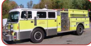
1984 PemFab/ E-One Pumper Detroit 8V92 Diesel Engine Automatic Transmission 1250 GPM Side-Mount Pump 750 Gallon Tank
