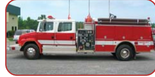
1993 Pierce/FL-80 Pumper Cummins 8.3L Diesel Engine Allison Automatic Transmission Waterous 1250 GPM Pump 1000 Gallon Steel Tank
