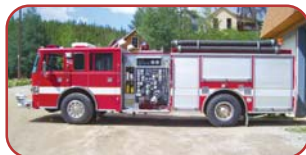
1995 Pierce Saber Rescue Pumper Detroit Diesel, Allison Automatic Waterous 1500 GPM Pump 750 Gallon Poly Tank 40 Gallon Poly Foam Tank
