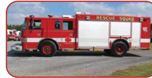
Pierce Lance Heavy Rescue Cummins 350 HP Diesel Engine Allison HT740 Automatic Light Tower, PTO Generator 12,000Lb Winch
