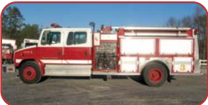
1996 Southern Coach Pumper Cummins 300HP Diesel Engine Allison MD3060P Automatic Hale 1000 GPM Side Mount Pump 1000 Gallon Poly Tank
