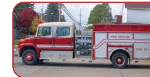
2002 ALF Rescue Pumper Cummins ISC 330 HP Diesel Allison MD3060P Automatic Hale 1500 GPM Side Mount Pump 750 Gallon Polypropylene Tank
