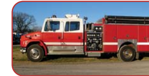
1996 Ferrara Rescue Pumper Cummins 300 HP Diesel Engine Allison Automatic Transmission Hale 1250 GPM Side Mount Pump 750 Gallon Poly Tank
