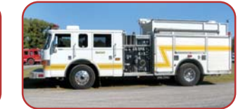
2001 Pierce Rescue Pumper Detroit Series 40E 330 HP Diesel Allison MD3060R Automatic Waterous 1500 GPM Pump 750 Gallon Poly Tank
