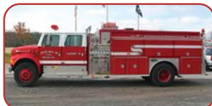
1992 E-One/Int'l Pumper/Tanker Cummins DT466 Diesel Allison MT643 Automatic Hale 1250 GPM Side-Mount Pump 1500 Gallon Poly Tank
