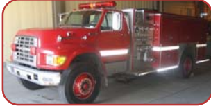
1995 E-One Commercial Pumper Diesel Engine, Automatic Transmission Ford F-800 Chassis Hale 1250 GPM Side-Mount Pump 1000 Gallon Polypropylene Tank
