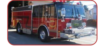
2002 Saulsbury Rescue Pumper Cummins Diesel, Allison Automatic Hale 1500 GPM Rear Mount Pump 500 Gallon Poly Tank Foam Pro Injection System
