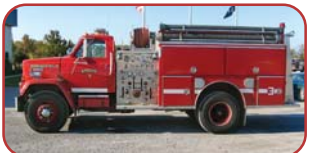
1986 E-One Commercial Pumper Detroit 6V71 Diesel Engine Allison Automatic Transmission Hale 1000 GPM Side-Mount Pump 1000 Gallon Poly Tank
