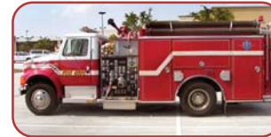
2000 Pierce/Int'l Commercial Rescue Pumper Cummins Diesel, Automatic Hale 1250 GPM Side-Mount Pump 750 Gallon Poly Tank
