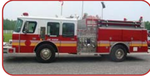
1988 E-One Cyclone Pumper Cummins Diesel Engine Allison Automatic Transmission Hale 1500 GPM Side Mount Pump 500 Gallon Poly Tank
