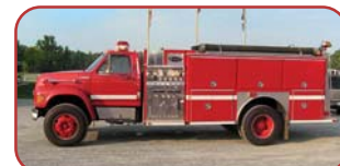
1998 E-One Commercial Pumper Cummins 250 HP Diesel Allison Automatic 1250 GPM Side-Mount Pump 1000 Gallon Poly Tank
