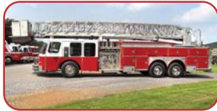
1988 E-One 95' Platform Detroit 8V92TA 475HP Diesel Allison HT740 Automatic Hale 1500 GPM Side Mount Pump 300 Gallon Aluminum Tank
