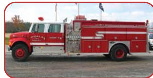
1992 E-One/Int'l Pumper/Tanker Cummins DT466 Diesel Allison MT643 Automatic Hale 1250 GPM Side-Mount Pump 1500 Gallon Poly Tank
