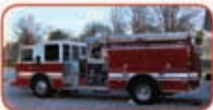
1997 Pierce Dash Rescue Pumper Detroit Series 40 Diesel Allison MD 3060 Automatic Waterous 1500 GPM Top-Mount Pump 500 Gallon Poly Tank
