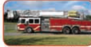
1991 E-One Hurricane 95' Platform Detroit 6V92TA 300 HP Diesel Allison MD3060 Automatic Hale QSMG 1250 GPM Pump 300 Gallon Poly Tank
