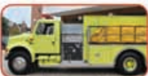
1991 Quality / International Tanker Int'l DT 466 - 245 HP Engine Automatic Transmission Waterous 500 GPM 2-Stage PTO Pump 1500 Gallon Fiberglass Tank Portable Dump Tank Rack
