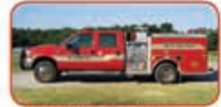
2000 KME Ford 4x4 Mini Pumper Hale 500 GPM Side Mount Pump 200 Gallon Tank Foam Pro Foam System 20 Gallon Class A Foam Cell
