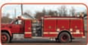
1997 Gatco / Ford Pumper Cummins 8.3L Diesel Engine Hale 1000 GPM Side-Mount Pump 1000 Gallon Poly Tank
