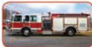
1997 Southern Coach Pumper Cummins C8.3 325 HP Diesel Allison MD 3060 Automatic Hale 1500 GPM Side-Mount Pump 750 Gallon Poly Tank
