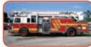
1996 Pierce Lance 75' Quint Detroit 8V92TA 500 HP Diesel Allison HD4060P Automatic Hale QSMG150 1500 GPM Pump 300 Gallon Poly Tank Onan 6KW Diesel Generator
