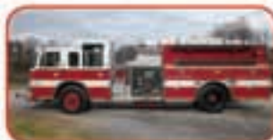
1996 Pierce Saber Pumper / Tanker Detroit Series 40 320 HP Diesel Allison MD3060 Automatic Waterous 1500 GPM Top-Mount Pump 1250 Gallon Poly Tank
