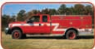
2003 Welch / F-550 4x4 Brush Truck Ford Diesel, Ford Automatic Waterous 400GPM Portable Pump 8&S 18 HP Pump Engine 220 Gallon Poly Tank 4-Bottle Cascade with Fill
