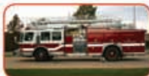
1995 E-One 50' Telesquirt Detroit 400 HP Diesel Allison Automatic Hale 1250 GPM Pump 300 Gallon Poly Tank A & B Foam System
