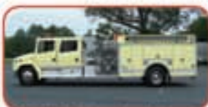
1996 KME / International Pumper Caterpillar Diesel Engine Allison MD3060 Automatic Hale 1500 GPM Top-Mount Pump 1000 Gallon Poly Tank
