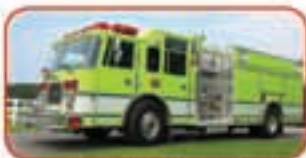
2000 Pierce Arrow Rescue Pumper Detroit 6V92TA 350 HP Diesel Allison HTB 741 Automatic Waterous CS 1250 GPM Pump 1000 Gallon Poly Tank Rockwood B2 400 GPM Foam System
