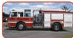
1998 Pierce Saber Rescue Pumper Detroit Series 40 Diesel Allison Automatic Transmission Waterous CSU 1500 GPM Pump 500 Gallon Poly Tank
