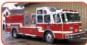
2000 E-One Cyclone II Rescue Pumper Cummins ISM Diesel, Allison Automatic Hale 1500 GPM Top-Mount Pump Enclosed Pump Panel 500 Gallon Poly Tank Foam Pro 2000 A&B Foam System
