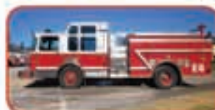
1992 Smeal / Spartan Rescue Pumper Cummins Diesel, Allison Automatic Waterous CSU 1500 GPM Enclosed Pump 900 Gallon Polypropylene Tank Rockwood ATP Foam System 30 Gallon Foam Cell
