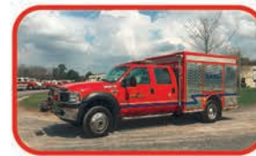
2007 Ford F-550 Quick Attack w/ CAFS Call for Custom Quote 125 GPM Pump 300 Gallon Tank, Foam 4x4
