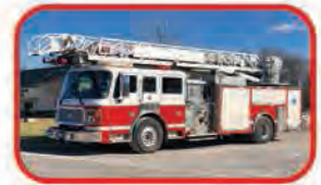
2002 Amercian LaFrance 75' Quint Hale 1500 GPM Pump 500 Gallon Tank Detroit Diesel
