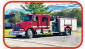
2004 Pierce Kenworth Pumper Waterous 1250 GPM Pump 1000 Gallon Tank Cummins Diesel
