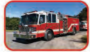
2005 Ferrara Igniter Rescue Pumper Waterous 1500 GPM Pump 500 Gallon Tank Detroit Diesel
