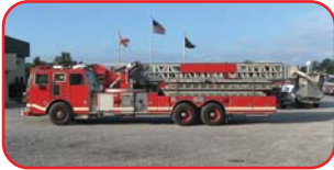
1993 Sutphen 100' Platform Cummins 410 HP Diesel Engine Allison Automatic Transmission 2 Monitors at Tip
