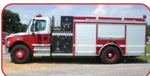
2004 ALF Pumper/Tanker Cat 3126 300 HP Diesel Allison Automatic Transmission ALF Power Flow 1250 GPM Pump 1250 Gallon Poly Tank
