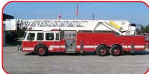
1994 Simon Duplex 102' Quint Detroit Series 60 475 HP Diesel Allison Automatic Transmission Waterous 2000 GPM Pump 250 Gallon Poly Tank
