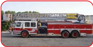
1995 E-One 95' Quint Detroit 8V92T Diesel Allison Automatic Hale QSMGT 1500 GPM Pump 200 Gallon Poly Tank
