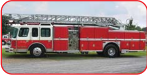
1990 E-One 75' Quint Detroit 8V92TA 450 HP Diesel Allison Automatic Transmission Hale CSD 150-22 1500 GPM Pump 400 Gallon Poly Tank
