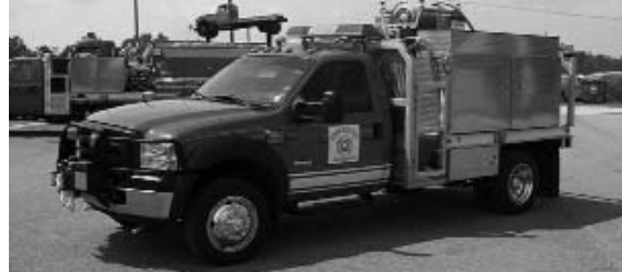
2007 F-550 Diesel 11' Flat Bed Brush Guard 375 CET Pump
