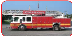
1995 E-One 110' Ladder Detroit 6V92TA Diesel Allison HT 740 Automatic Piped Waterway 8KW PTO-Driven Generator
