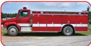
1995 Freightliner/Smeal Walk-Around Heavy Rescue Cummins Diesel Allison Automatic Honda 5KW Gas Generator
