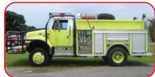
1998 Int'l 4x4 Interface Pumper Navistar DT466 Diesel Allison Automatic Transmission Hale 500 GPM Side-Mount Pump 500 Gallon Poly Tank Robwen Foam System
