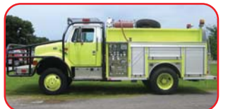
1998 Int'l 4x4 Interface Pumper Navistar DT466 Diesel Allison Automatic Transmission Hale 500 GPM Side-Mount Pump 500 Gallon Poly Tank Robwen Foam System
