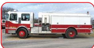
1988 Wolverine Pumper/Tanker Detroit 8V92TA Diesel Allison HT740 Automatic Hale QSMG 1500 GPM Pump 1200 Gallon Steel Tank
