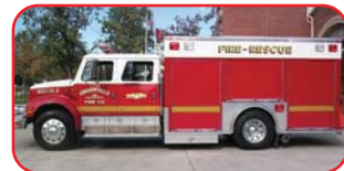
1993 International Heavy Rescue Int'l Diesel, Allison Automatic Winco 20KW PTO Generator Amkus Simo Pump SuperVac Command Light 6000psi DOT 8-Bottle Cascade
