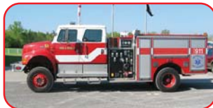
2000 Pierce 4x4 Interface Pumper Navistar DT466E 300 HP Diesel Allison MD 3060 Automatic Waterous 500 GPM Pump 500 Gallon Poly Tank
