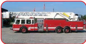
1994 Simon Duplex 102' Quint Detroit Series 60 475 HP Diesel Allison Automatic Transmission Waterous 2000 GPM Pump 250 Gallon Poly Tank
