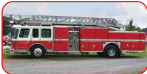
1990 E-One 75' Quint Detroit 8V92TA 450 HP Diesel Allison Automatic Transmission Hale CSD 150-22 1500 GPM Pump 400 Gallon Poly Tank
