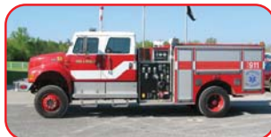
2000 Pierce 4x4 Interface Pumper Navistar DT466E 300 HP Diesel Allison MD 3060 Automatic Waterous 500 GPM Pump 500 Gallon Poly Tank
