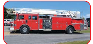
1990 Pierce Lance 75' Quint Cummins 400 HP Diesel Engine Allison HT-740 Automatic Waterous 1500 GPM Pump 300 Gallon Steel Tank
