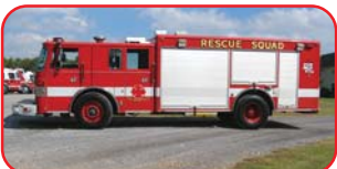
1992 Pierce Lance Heavy Rescue Cummins 350 HP Diesel Engine Allison HT740 Automatic Light Tower, PTO Generator 12,000Lb Winch
