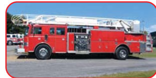
1990 Pierce Lance 75' Quint Cummins 400 HP Diesel Engine Allison HT-740 Automatic Waterous 1500 GPM Pump 300 Gallon Steel Tank
