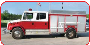
1997 Freightliner/Westex Rescue Cummins 8.3L Diesel Allison Automatic Hale AP50-20 500 GPM Pump 350 Gallon Aluminum Tank
