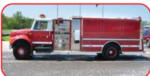
1993 Int'l/Central Pumper/Tanker Navistar Diesel, Allison Automatic Hale 1250 GPM Side-Mount Pump 1300 Gallon Poly Tank Feecon Around-the-Pump Foam System
