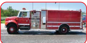
1993 Int'l/Central Pumper/Tanker Navistar Diesel, Allison Automatic Hale 1250 GPM Side-Mount Pump 1300 Gallon Poly Tank Feecon Around-the-Pump Foam System
