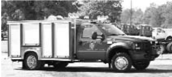
2007 F-550 Diesel 11' Rescue Body, 300 Gal Water, CAFS, Generator, Roll Up Doors
