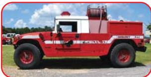
1994 Hummer 4x4 Brush Truck General Motors 6.5L Diesel Automatic Transmission Darley 2BE1A Independent Pump 200 Gallon Poly Tank
