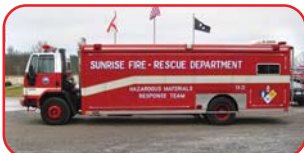
1989 Ford/Hackney Heavy Rescue/Hazmat Interior Command Center in Rear Ford Diesel, Allison Automatic Onan 7.5KW Hydraulic Generator Light Tower with 2 -1500W Lights
