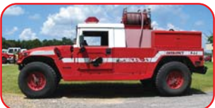
1994 Hummer 4x4 Brush Truck General Motors 6.5L Diesel Automatic Transmission Darley 2BE1A Independent Pump 200 Gallon Poly Tank
