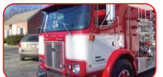
1982 Pierce Pumper/Tanker Cummins 300 HP Diesel Fuller 6-speed Manual Waterous 1500 GPM Pump 1500 Gallon Steel Tank
