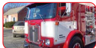
1982 Pierce Pumper/Tanker Cummins 300 HP Diesel Fuller 6-speed Manual Waterous 1500 GPM Pump 1500 Gallon Steel Tank
