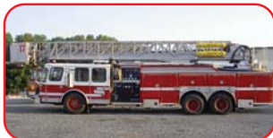
1995 E-One 95' Quint Detroit 8V92T Diesel Allison Automatic Hale QSMGT 1500 GPM Pump 200 Gallon Poly Tank
