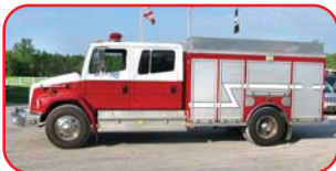
1997 Freightliner/Westex Rescue Cummins 8.3L Diesel Allison Automatic Hale AP50-20 500 GPM Pump 350 Gallon Aluminum Tank
