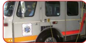
1991 E-One Cyclone Tilt Cab Detroit Diesel Engine Allison Automatic Transmission Hale 1500 GPM Pump 750 Gallon Poly Tank
