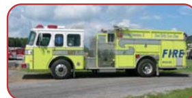
1990 E-One Hush Custom Pumper Detroit Diesel, Allison Automatic Hale 1500 GPM Top Mount Pump 500 Gallon Polypropylene Tank
