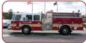
1989 E-One Cyclone Pumper Cummins LTA-10 300 HP Diesel Allison HT740 Automatic Hale 1500 GPM Side Mount Pump 500 Gallon Poly Tank
