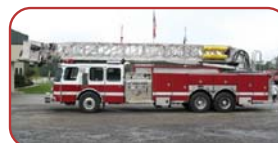
1995 E-One 95' Platform Detroit 8V92TA Diesel Engine Allison Automatic Transmission Hale 1500 GPM Side Mount Pump 300 Gallon Polypropylene Tank
