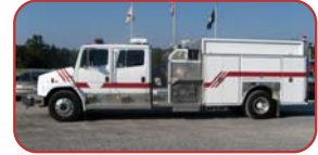
1997 E-One/Freightliner Commercial Pumper Cummins Diesel, Allison Automatic Hale 1250 GPM Pump 700 Gallon Poly Tank
