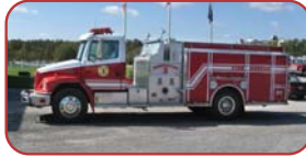
1998 Freightliner/ RD Murray Commercial Pumper Cummins Diesel, Allison Automatic Hale 1000 Gallon Top-Mount Pump 500 Gallon Poly Tank
