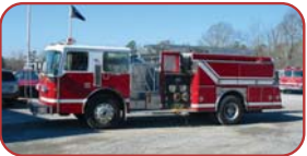
1989 American Eagle/Duplex Pumper Detroit Diesel, Automatic Transmission Hale 1500 GPM Top Mount Pump NEW 1000 Gallon Poly Tank
