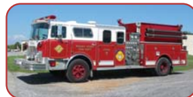
1991 Ward/Mack Pumper Mack Diesel, Allison Automatic Waterous CMU 1500 GPM Pump 750 Gallon Steel Tank
