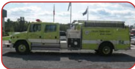
95 Pierce Commercial Pumper Freightliner FL80 Chassis Cummins Diesel, Allison Automatic Hale 1250 GPM Pump 1000 Gallon Poly Tank
