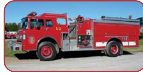
1988 Smeal C-8000 Pumper Ford C-8000 Chassis Caterpillar Diesel, Allison Automatic Waterous 1250 GPM Pump 750 Gallon Steel Tank
