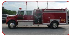
1992 Southern Coach Commercial Pumper International Diesel, Allison Automatic American Godiva 1000 GPM Pump 750 Gallon Fiberglass Tank
