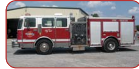
1988 American Eagle/ Spartan Pumper Detroit Diesel, Allison Automatic Hale 1750 GPM Pump 750 Gallon Poly Tank
