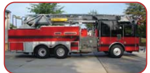
2004 HME 75' Quint HME 1871 Series Chassis Cummins Diesel, Allison Automatic Hale 1500 GPM Pump 650 Gallon Poly Tank
