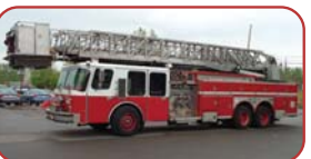
1988 E-One 95' Platform Quint Detroit 475 HP Diesel Allison Automatic Hale 1500 GPM Side Mount Pump 300 Gallon Aluminum Tank
