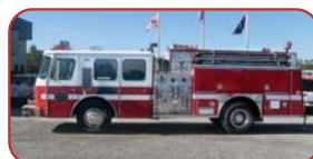
1990 E-One Cyclone Custom Pumper Cummins Diesel, Allison Automatic Hale 1500 GPM Side Mount Pump 750 Gallon Poly Tank
