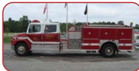
1995 E-One Commercial Pumper Freightliner FL80 Four Door Chassis Cummins Diesel, Allison Automatic Hale 1250 GPM Pump 750 Gallon Poly Tank
