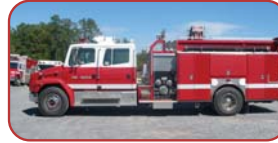
1997 Ferrara FL80 Commercial Pumper Cummins Diesel, Allison Automatic Hale 1250 GPM Pump 750 Gallon Poly Tank
