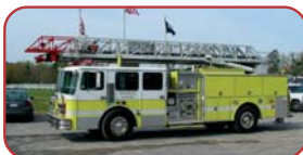
1987 KME 75' Quint Detroit Diesel, Allison Automatic Waterous CSU 1500 GPM Pump 300 Gallon Fiberglass Tank Akron Foam Eductor
