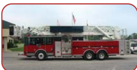
1999 Pierce Sky Arm 3D Paramount VI Body International Diesel, Ford Automatic Hale 1500 GPM Pump 300 Gallon Tank
