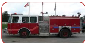
1997 E-One Cyclone II Pumper Detroit Diesel, Allison Automatic Hale 1250 GPM Pump 500 Gallon Poly Tank
