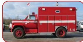
1990 E-One Walk-In Rescue GMC 7000 Chassis General Motors Diesel Engine Allison AT545 Automatic 1000 Watt Inverter
