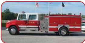
1997 Freightliner/Ferrara FL80 Commercial Pumper Cummins Diesel, Allison Automatic Hale 1250 GPM Pump New 1000 Gallon Poly Tank
