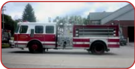
1989 E-One Hurricane Pumper Diesel Engine Automatic Transmission 1250 GPM Pump 1000 Gallon Poly booster tank
