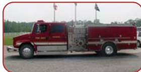
1994 Boardman Commercial Pumper Cummins Diesel, Allison Automatic Waterous 1500 GPM Pump 1000 Gallon Poly Tank
