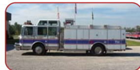
1989 Spartan Rescue Spartan Gladiator Vista Cab Interior: Command Center Cummins 350 Horsepower Diesel Engine Allison Automatic Transmission
