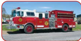
1989 Ward/Mack Pumper Mack Diesel, Allison Automatic Waterous CMU 1500 GPM Pump NEW 1000 Gallon Poly Tank
