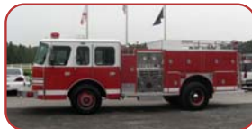
1991 E-One Protector Custom Pumper Cummins Diesel, Allison Automatic Hale 1000 GPM Pump 500 Gallon Aluminum Tank
