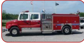
1998 E-One/Freightliner Commercial Pumper Cummins Diesel, Allison Automatic Hale 1250 GPM Pump New 1000 Gallon Poly Tank
