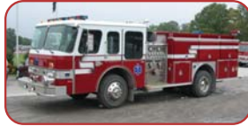
1987 E-One Hush Pumper Detroit Diesel, Allison Automatic Hale 1500 GPM Side Mount Pump 500 Gallon Aluminum Tank
