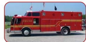
1988 E-One Heavy Rescue Detroit 8V92TA Diesel Engine Allison Automatic Transmission Command Desk and Radio Center 6 - 500 Watt Quartz Lights
