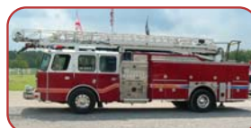
1997 E-One 75' Quint Detroit Diesel, Allison Automatic All Aluminum Cab, Body, and Ladder 1500 Gallon Pump, 400 Gallon Tank 1000 GPM Nozzle at Tip
