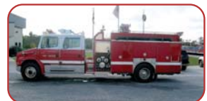
1994 Ferrara FL80 Pumper Freightliner FL80 4-Door Cab Cummins Diesel, Allison Automatic Hale 1250 GPM Pump 750 Gallon Poly Tank
