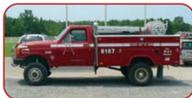
1990 Marko 4x4 Quick Attack Int'l Diesel, Ford Automatic 90 GPM Gasoline Powered Pump 200 Gallon Polypropylene Tank
