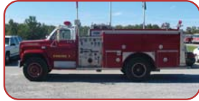
1986 Chevy C70 Pumper Detroit 8.2 Liter Diesel Engine Allison Automatic Transmission Hale 1000 GPM Pump 500 Gallon Aluminum Tank
