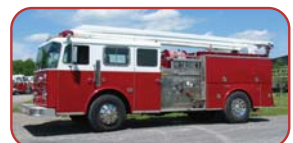
1989 Seagraves 54' Telesquirt Detroit Diesel, Allison Automatic Waterous 1250 GPM Pump 500 Gallon Steel Tank
