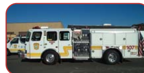
2000 E-One Pumper Hale 1500 GPM Pump 750 Gallon Poly Tank Akron ATP 125 Foam System 20 Gallon Foam Tank
