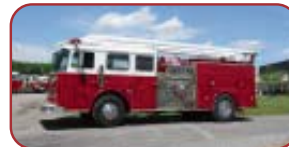
1989 Seagraves 54' Telesquirt Detroit Diesel, Allison Automatic Waterous 1250 GPM Pump 500 Gallon Tank $69,000
